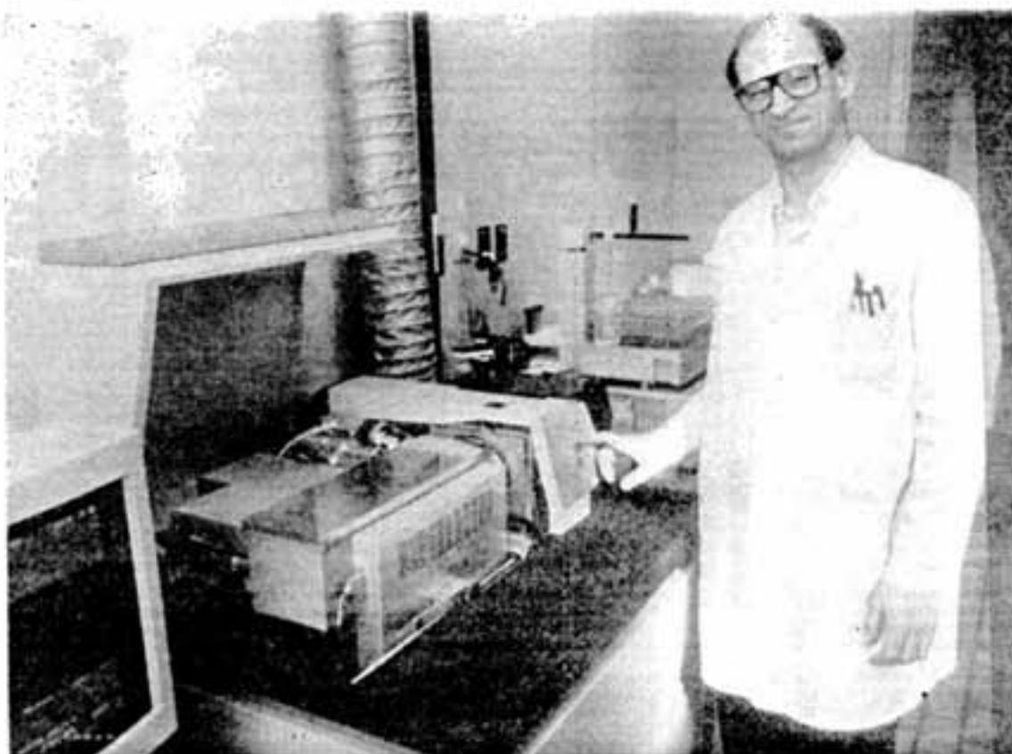
Development chemist Zbig Waszczylo works the ICP Mass Spectrometer which allows chemists to study the quality of Inco's nickel in greater detail — even as low as parts per trillion.
