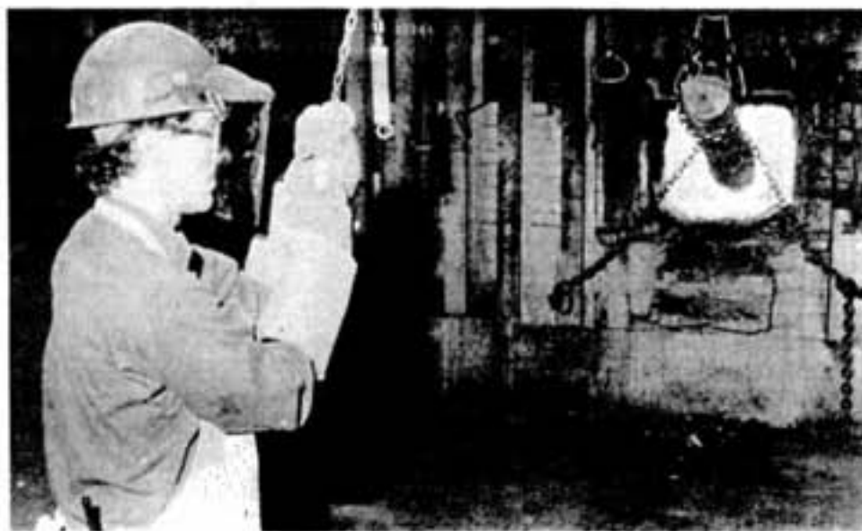
Furnace crew employees, including Ray Morin, right, position a hardwood pole for placing into one of two anode furnaces at the Copper Refinery. The poles are submerged about two feet into the copper matte and burn quickly in temperatures of about 2,200°F.
