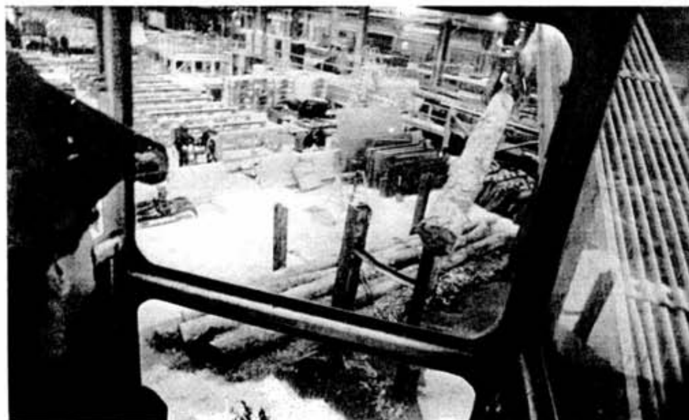
Ray Morin, head furnaceman with 28 years service at Inco, operates a crane to unload the logs from a pile before they are inspected by employees and hoisted into the anode furnaces.
