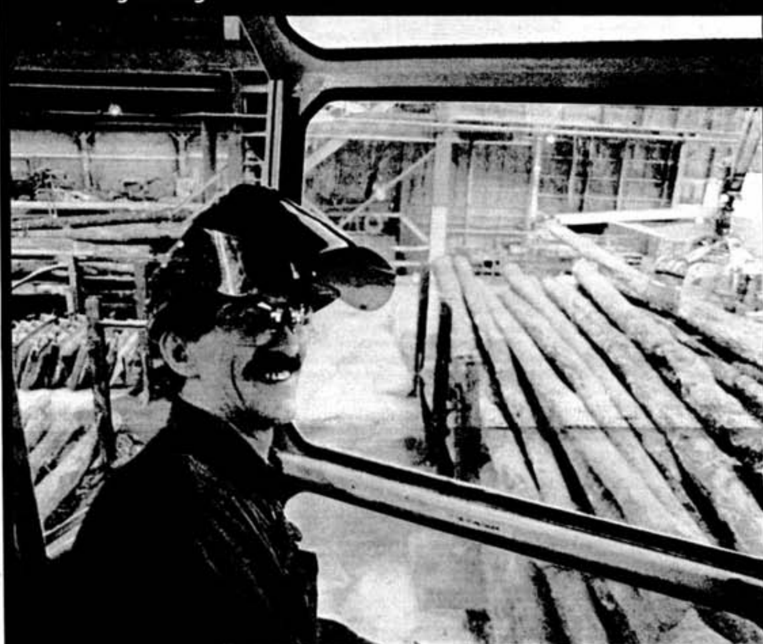
From his perch inside the cab of an overhead crane, Copper Refinery furnaceman Ray Morin has a good view of the logs destined for the anode furnaces where they are used to burn off oxygen in copper matte. A project to improve the quality of the logs has resulted in savings of $85,000 annually. Read more about the project in the story at the bottom of this page.
