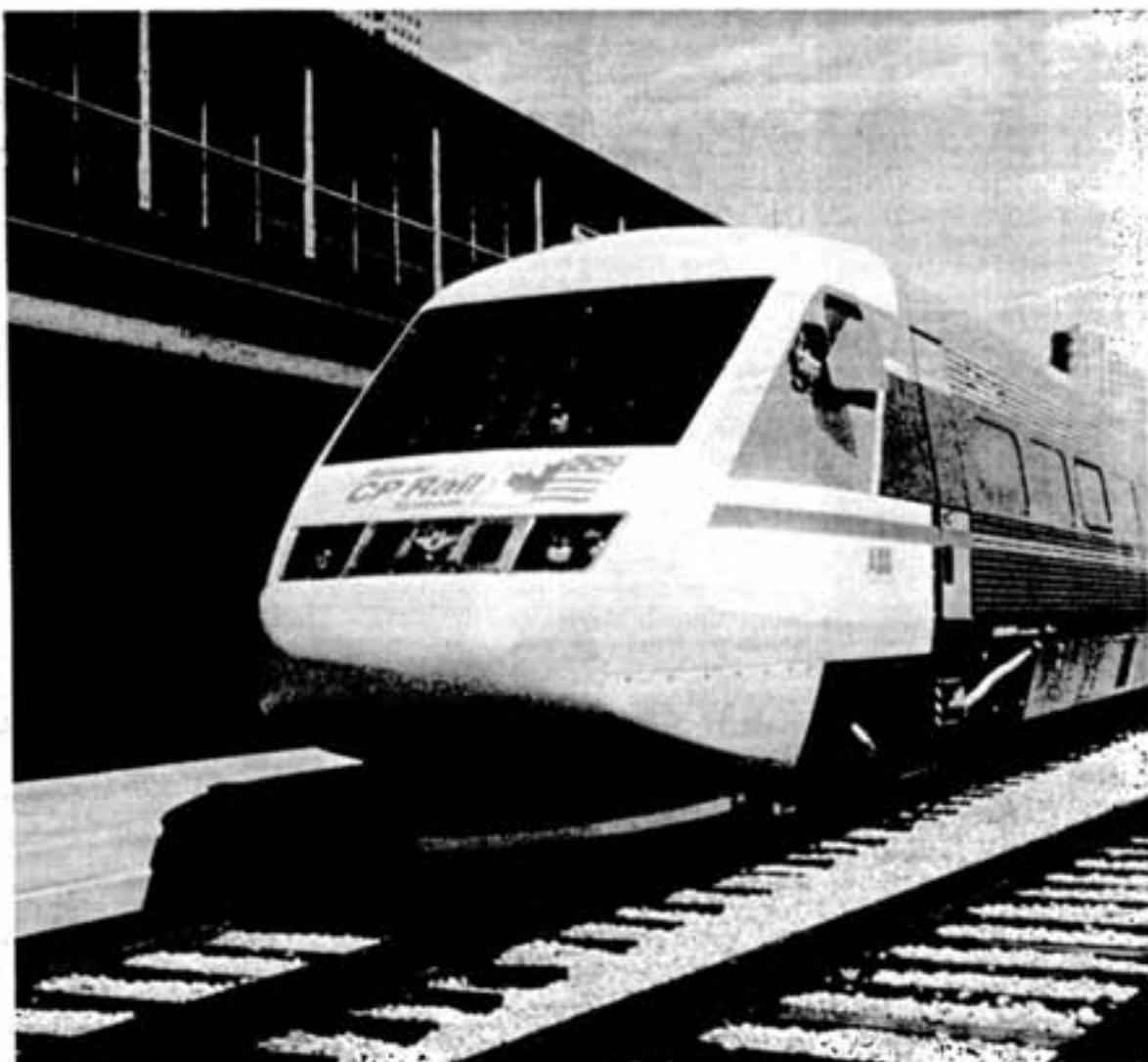
The X-2000 train uses nickel stainless steel in structural members and exterior sheathing.
