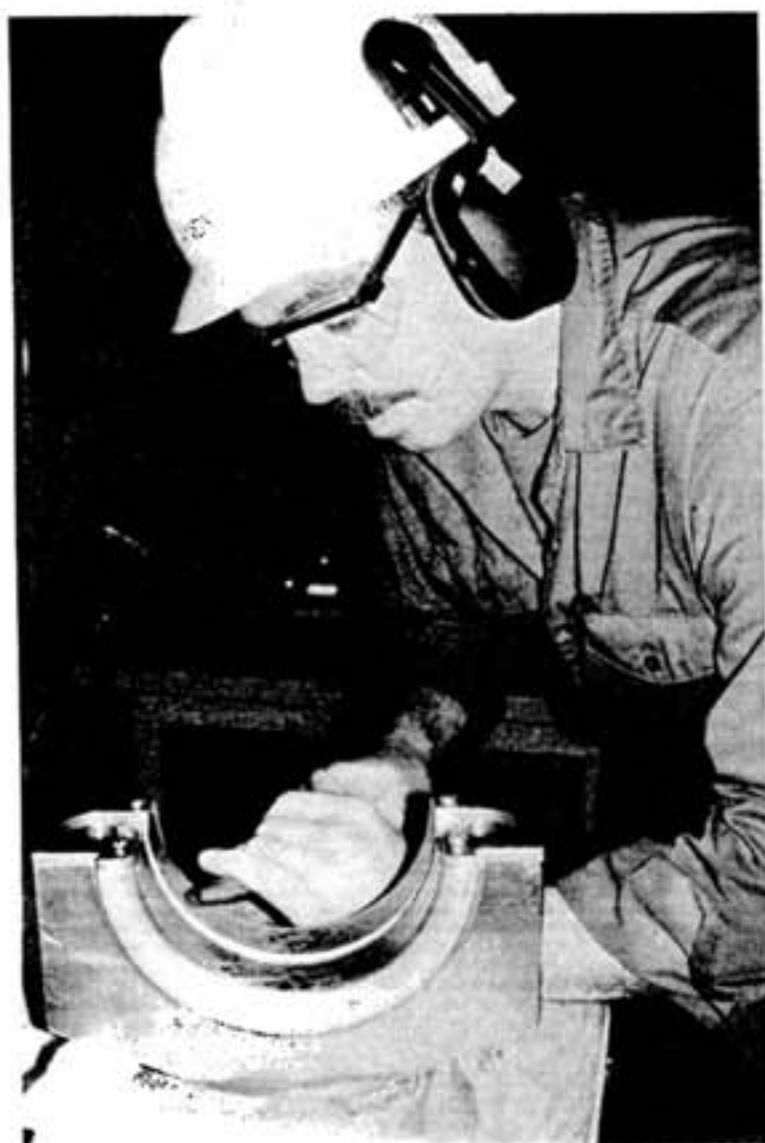
Machinist Andy Bazinet scrapes a babbitt bearing from the #3 high pressure oxygen compressor at the Oxygen Plant. The compressor is currently undergoing a major overhaul.
