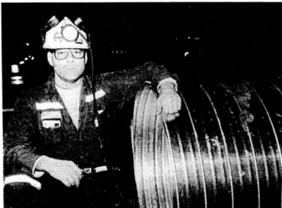
Ron Stewart, ventilation technician at Stobie Mine, is impressed with the new ventilation tubing made underground. "We're having our ventilation manufactured underground. Before we had it made on surface in shops around Sudbury. But you could only ship two of them down at a time because they were three feet wide and 10 feet long. So what we can make in a day would have taken a month to get underground."
