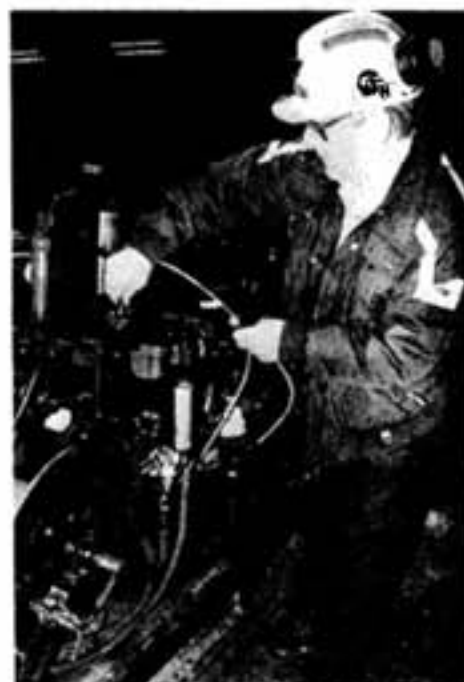
Rick Bourget, geological technician at Copper Cliff North Mine, hooks up the metal detector to the computer mounted on the diesel-powered double-track probe cart during a test on surface. The probe relays a reading to the computer every foot along a 400-foot drill hole, revealing whether it detects ore or rock from inside the hole.
