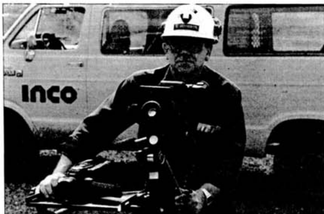
Gordon Roberts, NDE specialist, uses a $60,000 infrared camera and associated equipment at a power substation at Copper Cliff South Mine. The camera detects heat as it scans transformers, lightning arresters and aerials. A hot or cool spot can indicate problem areas that need maintenance and/or replacement before safety or production is affected.
