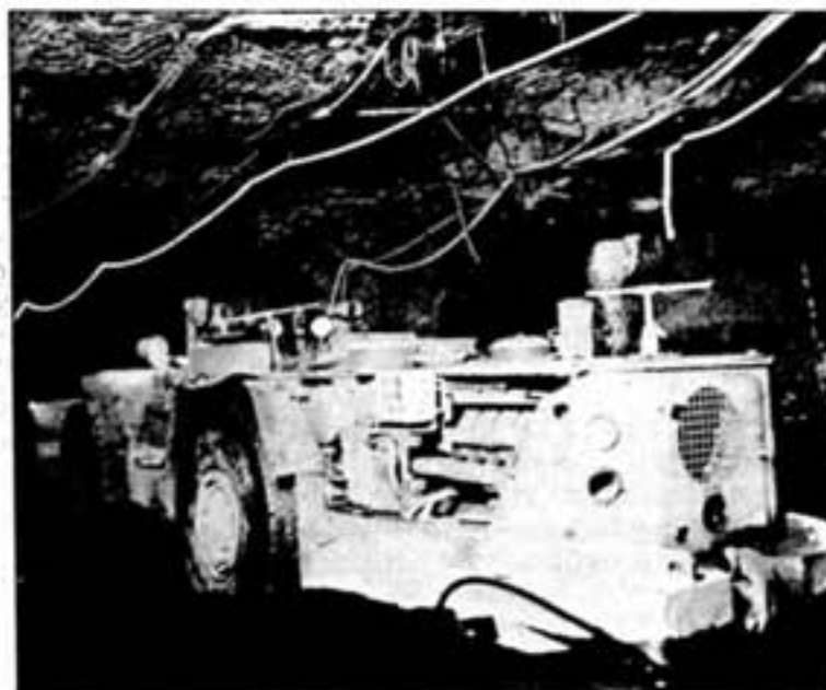
An overhead light track serves as a guidance system for the automated roboscoop while an operator on surface controls its movements.
