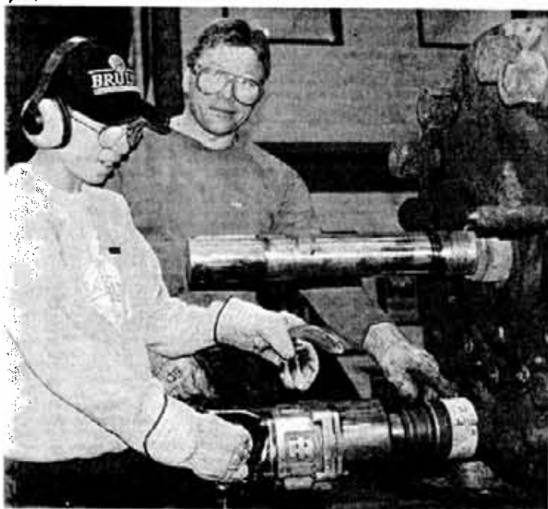
Ed Wolski gives son Jonathan, 14, a few tips on handling an impact wrench to remove rods from an 11-stage mine dewatering pump.
