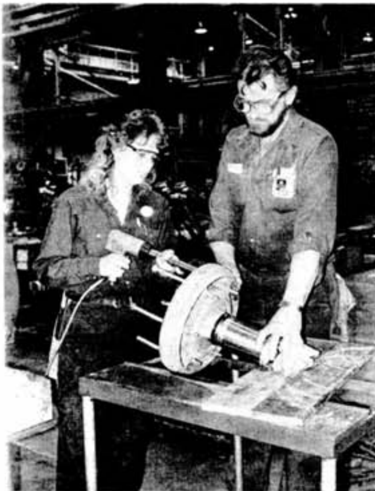
With a steady hand from machinist/instructor Ron Ylitalo, Lynne Descary tightens the nuts on the oil housing bottom of a submersible pump under repair at Div Shops.
