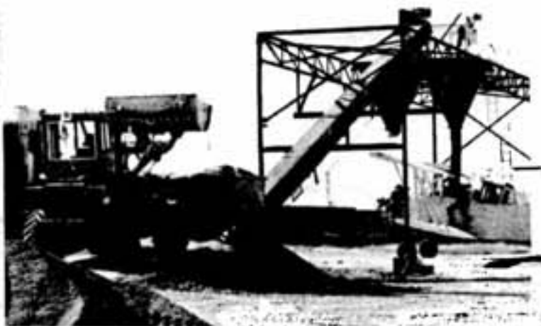
A tractor, bin of lime, conveyor and overhead loading facility help keep the aircrafts' time on the ground to under two minutes.
