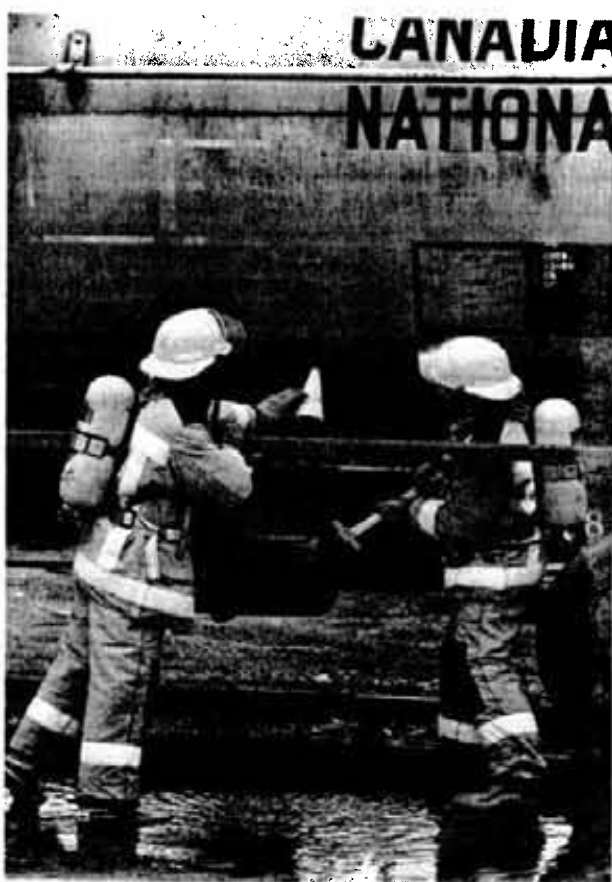
Sudbury firemen plug up a hole in the tank car, then (right) place a patch on it.
