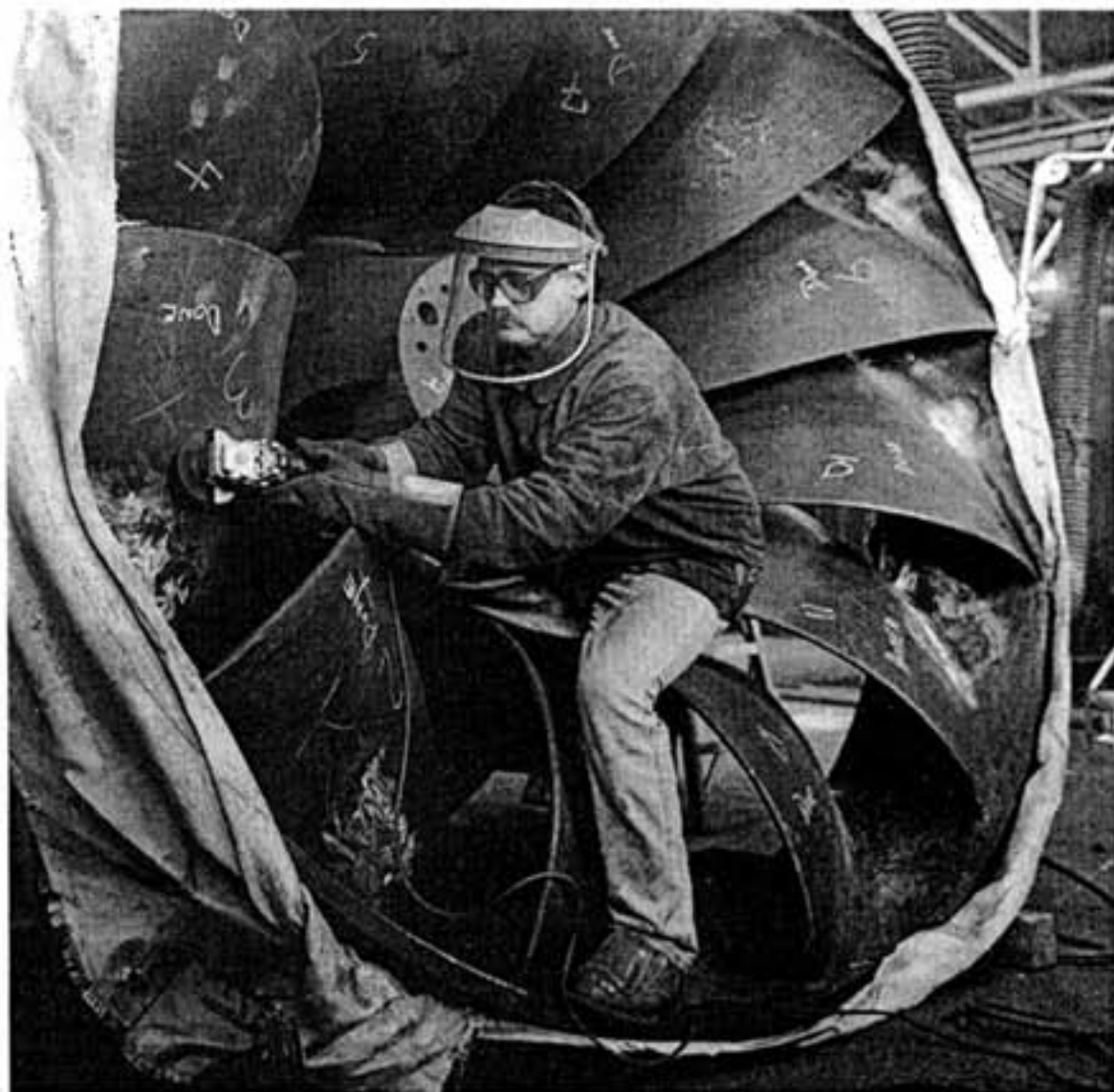
Welder Ray Higgs is dwarfed by the cast iron waterwheel he's repairing.
