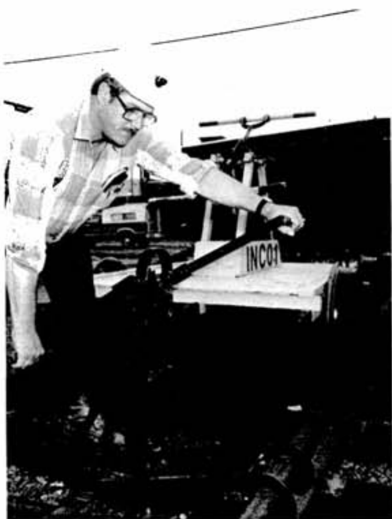
Track maintenance supervisor Ray Bromley checks a hand-operated drill and hand pump car to ensure the antique equipment is still in good operating order. The restored equipment is on display in front of the Transportation offices at the Smelter Complex.
