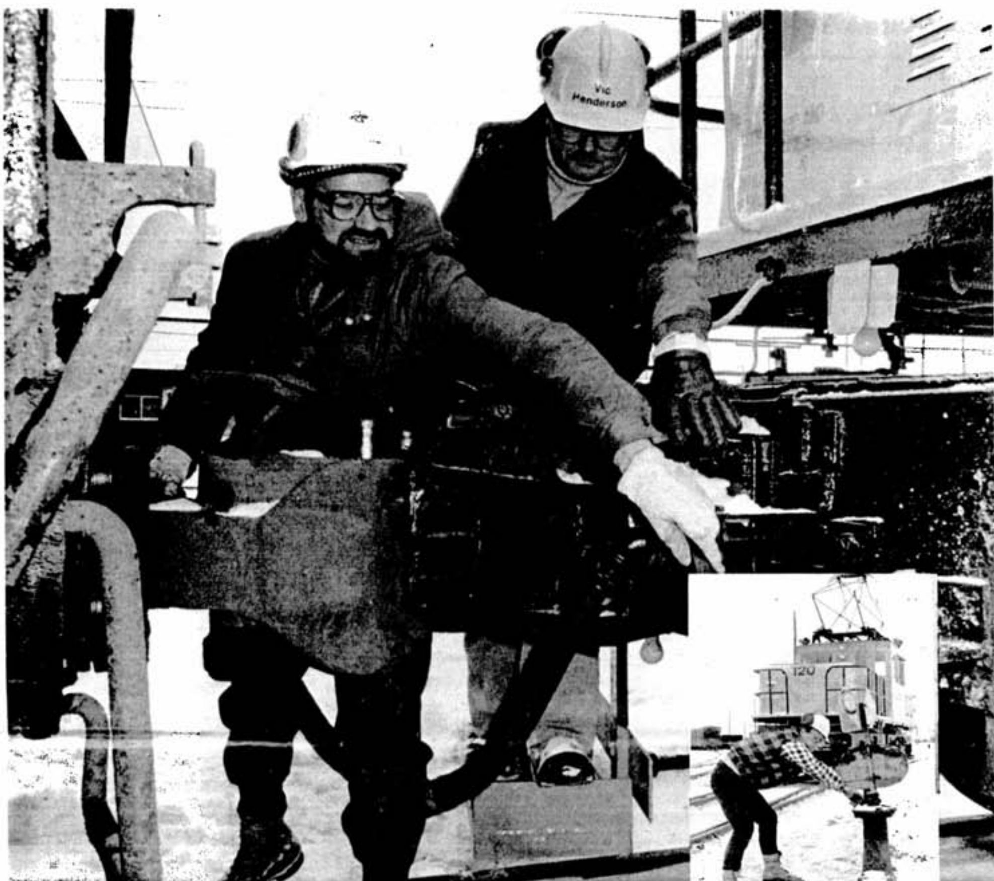
George Canapini learns to unhook a car from a locomotive. Doing the instructing is Vic Henderson (right). Putting his back into the switch while the locomotive waits for his signal to proceed is Joe Nicholls.
