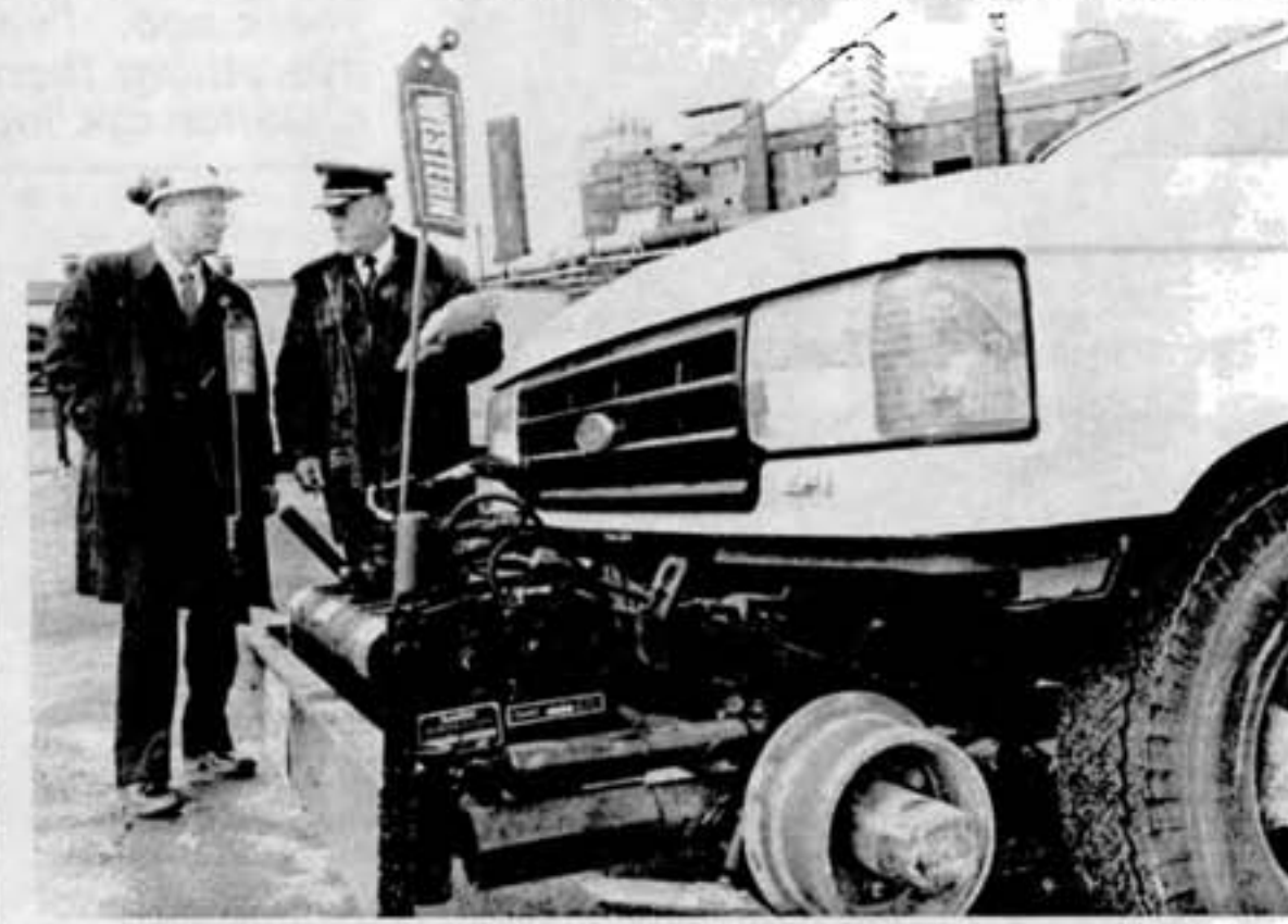
Safety and Training manager Dar Anderson and Sudbury Fire Chief Don McLean take a look at the rail-riding equipment housed on the front of the truck.
