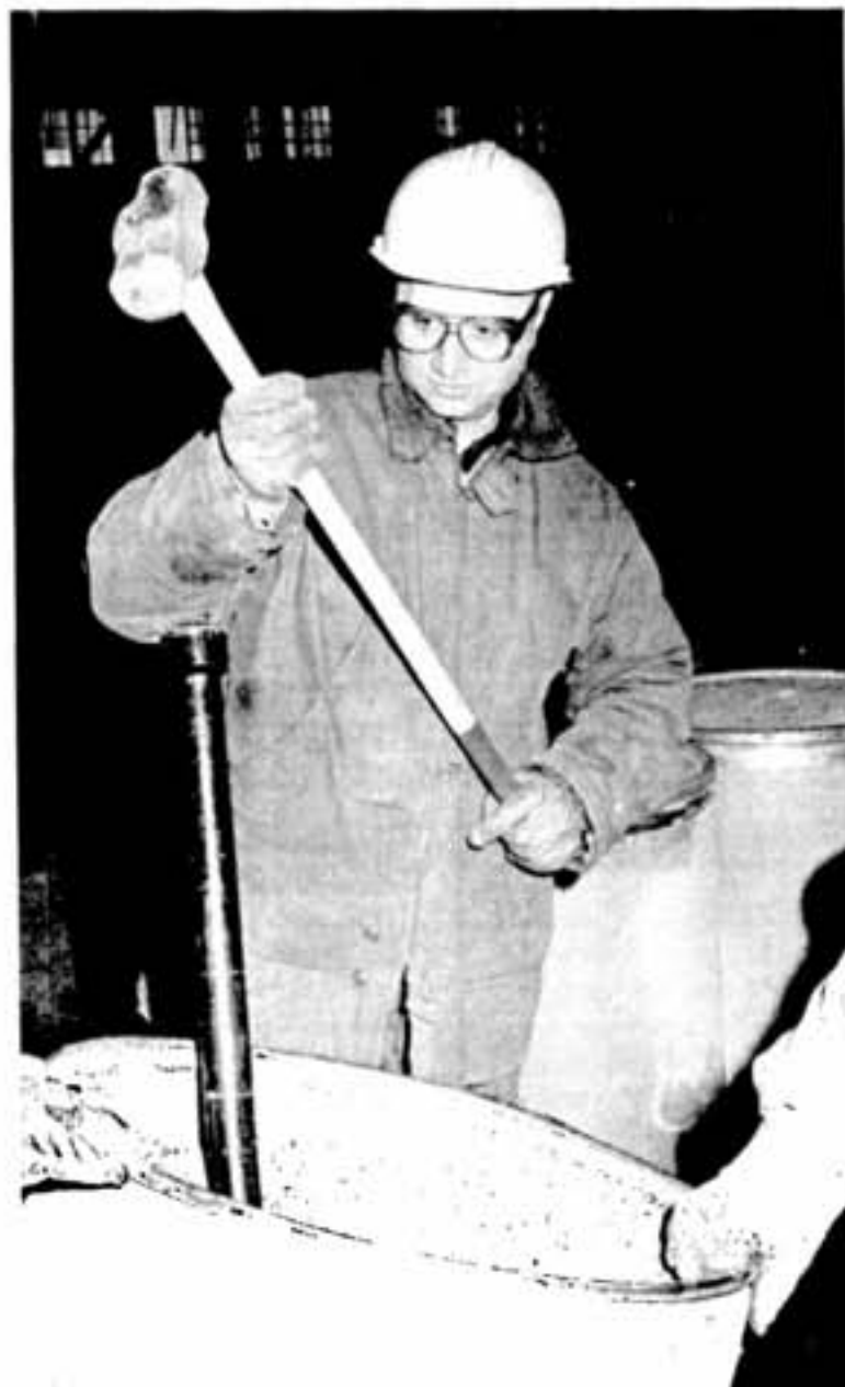
Another few blows with the sledge hammer and the sample pipe is ready for removal, filled with the catalyst material.
