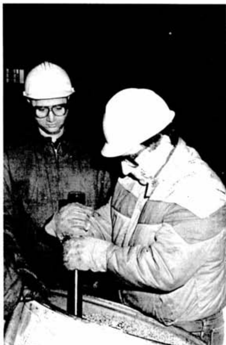
Yvon Lepage works the pipe around in the material in order to get a better sample while Len Incerti waits with the sledge.
