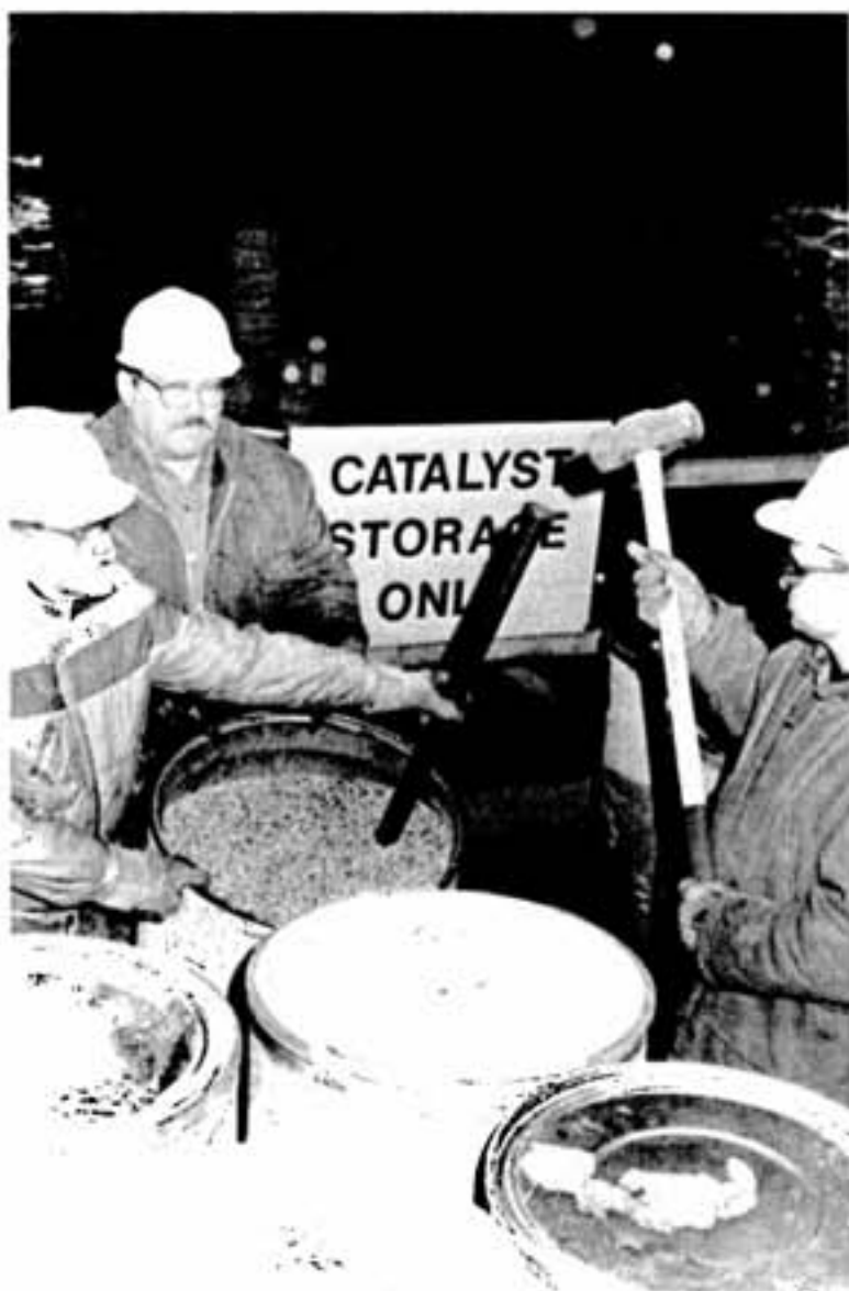
Yvon Lepage, Len Incerti and Art Maestrello drive a sampling pipe into the catalyst material.
