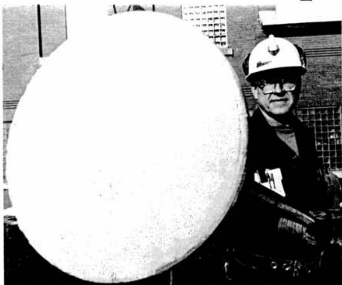
The cone-shaped charge, adapted to mining use by the pole holder on the apex.
