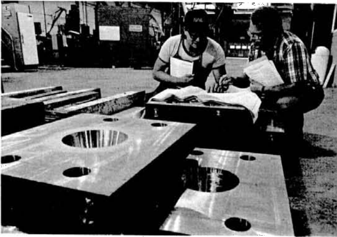
Welder Steve Reynolds and shop supervisor Bernie Piche plan welds on copper pieces.
