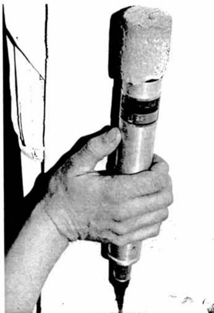
The geophone, shown above, is a monitoring device used underground to detect microseismic activity.
