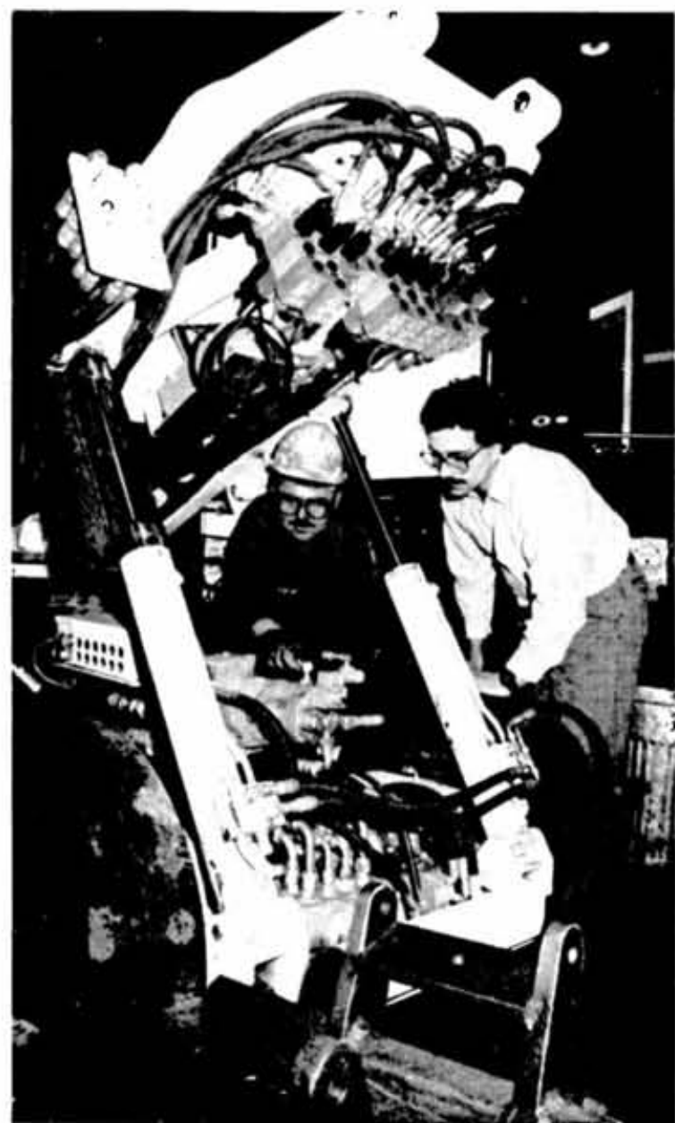
Equipment assembler Richard Lachance, left, and Mines Research engineer Frank Catalano examine a new one-man diamond drill under construction at North Mine.
