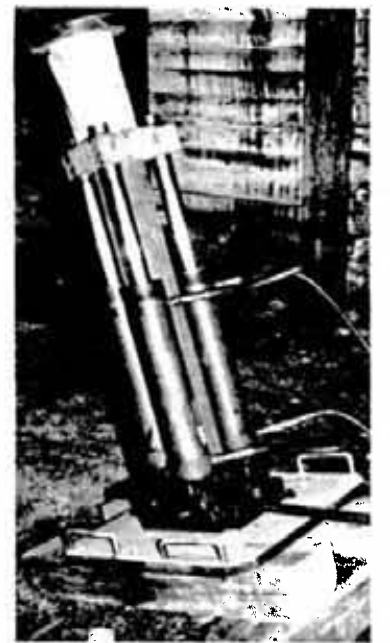
As the pistons extend, rod (centre of four pistons) is eased out of the hole.
