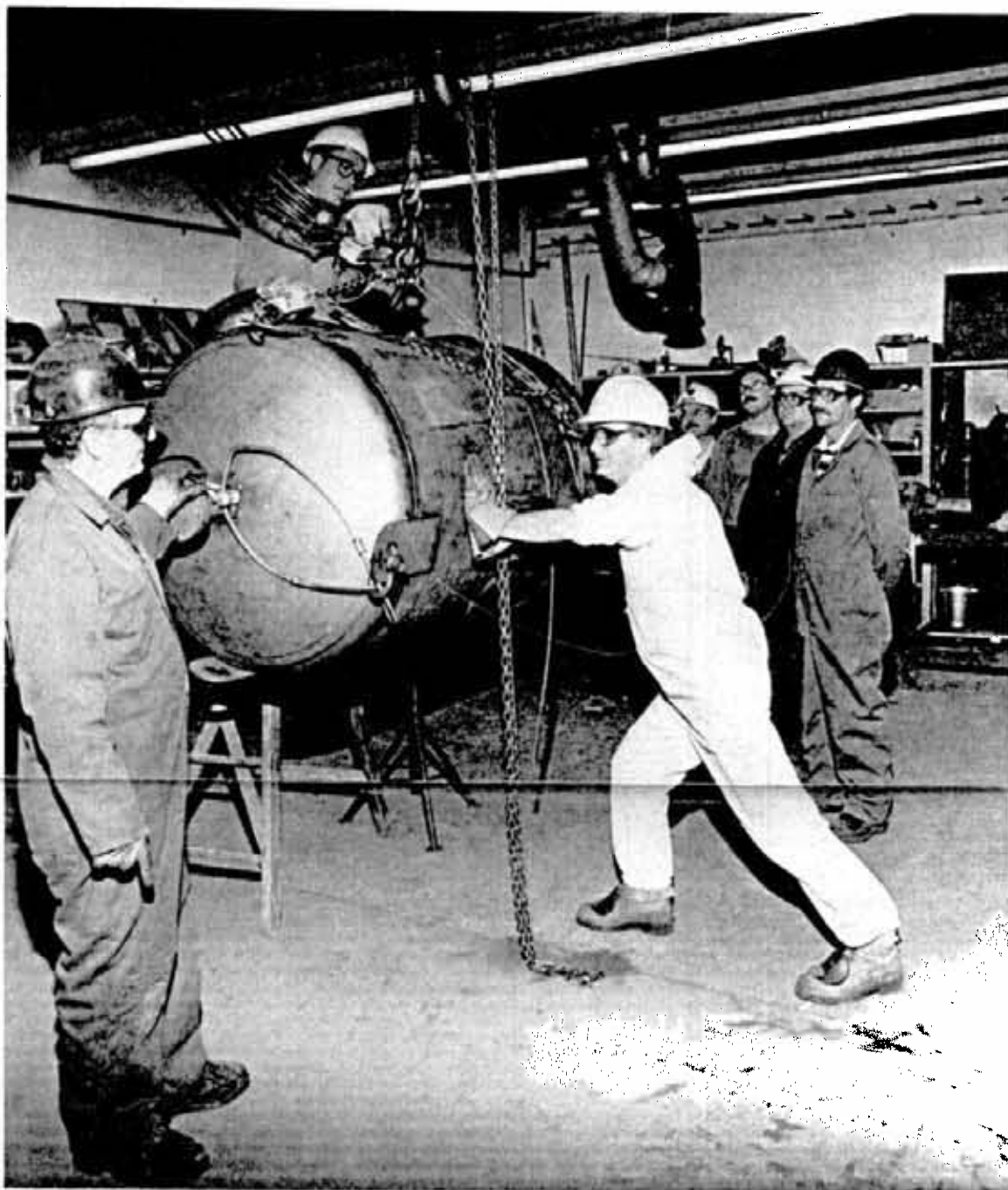
Rigger leader George Lebeau watches as crew Wayne Kerr (top) and Gerry Taillefer rehearse "drifting" a tank as part of their maintenance mechanic apprenticeship training.
