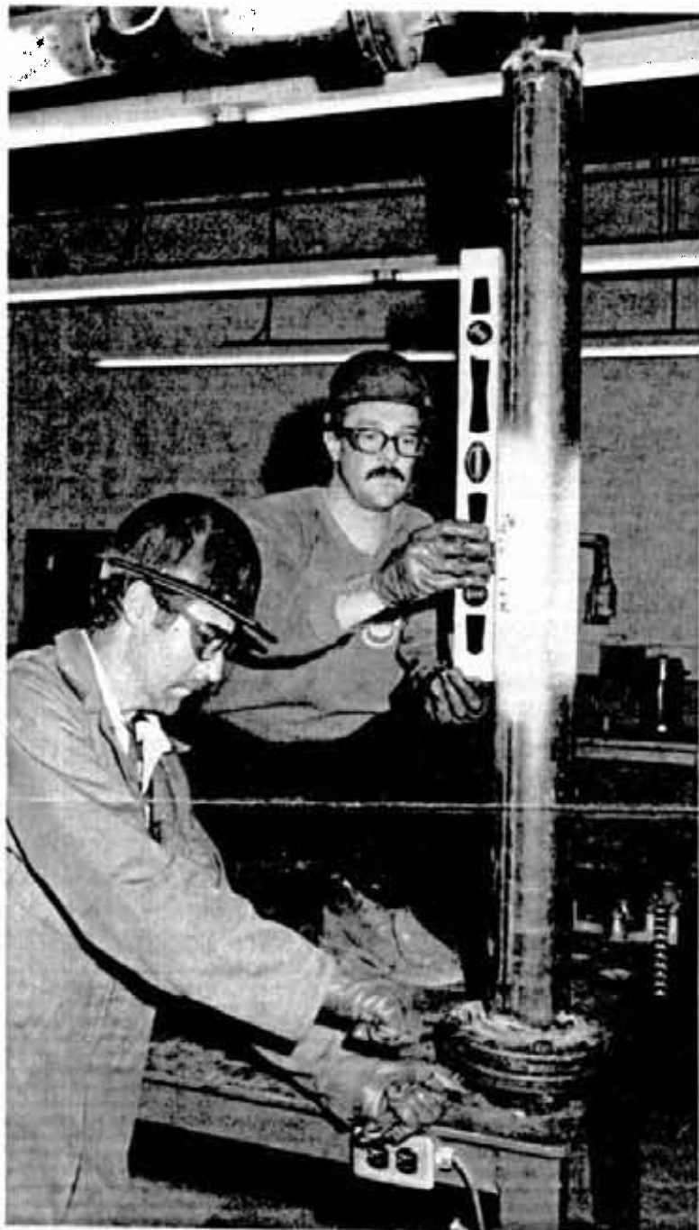
Glen Eady checks the level while Wilfred Budgell tightens the bolt in welded pipe section, a procedure that's part of Inco's apprenticeship training.
