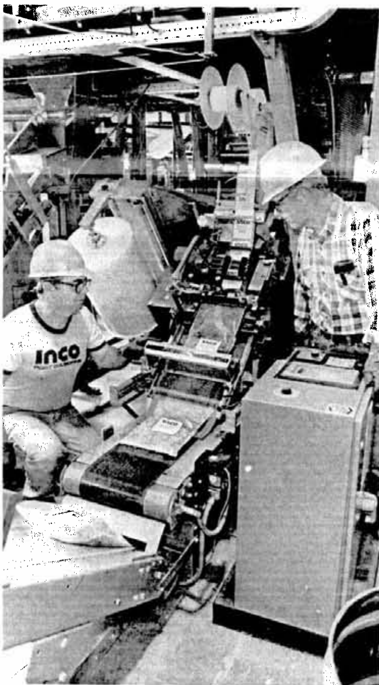
Orazio Nuccitelli, left, and his brother, Mario, bring 64 years of Inco experience with them in running the Port Colborne Refinery's new 10-kilo packaging system for handling nickel rounds.
