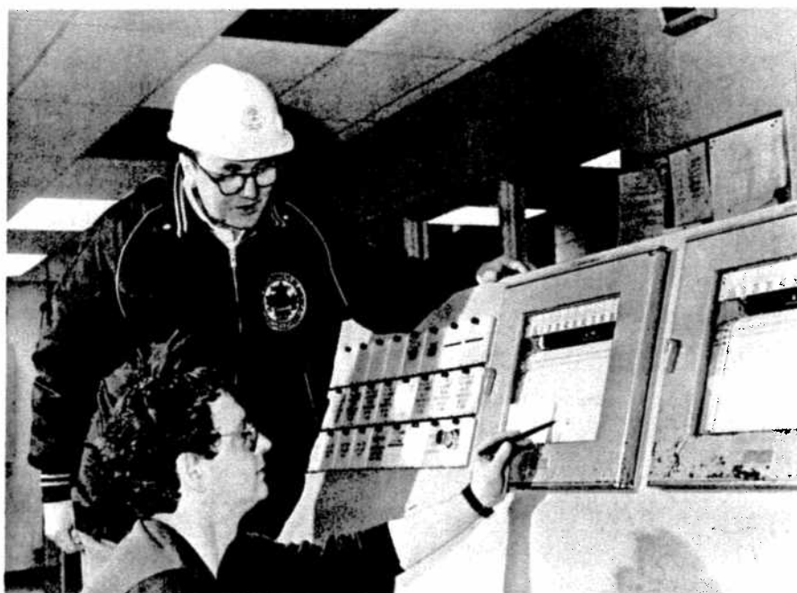
Worker safety rep. Ray Vallee, and control room operator, Del Thompson, check out a carbonyl monitor in the nickel refinery control room. The monitor would alert the control room operator if there was a leak of potentially dangerous carbonyl gas which is used in the refining process at the nickel refinery.
