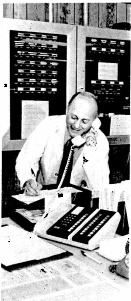
Ron Smith, a plant protection officer at No. 1 First Aid, demonstrates the use of a sophisticated phone hook-up which will automatically activate up to 16 other phones with one call.
