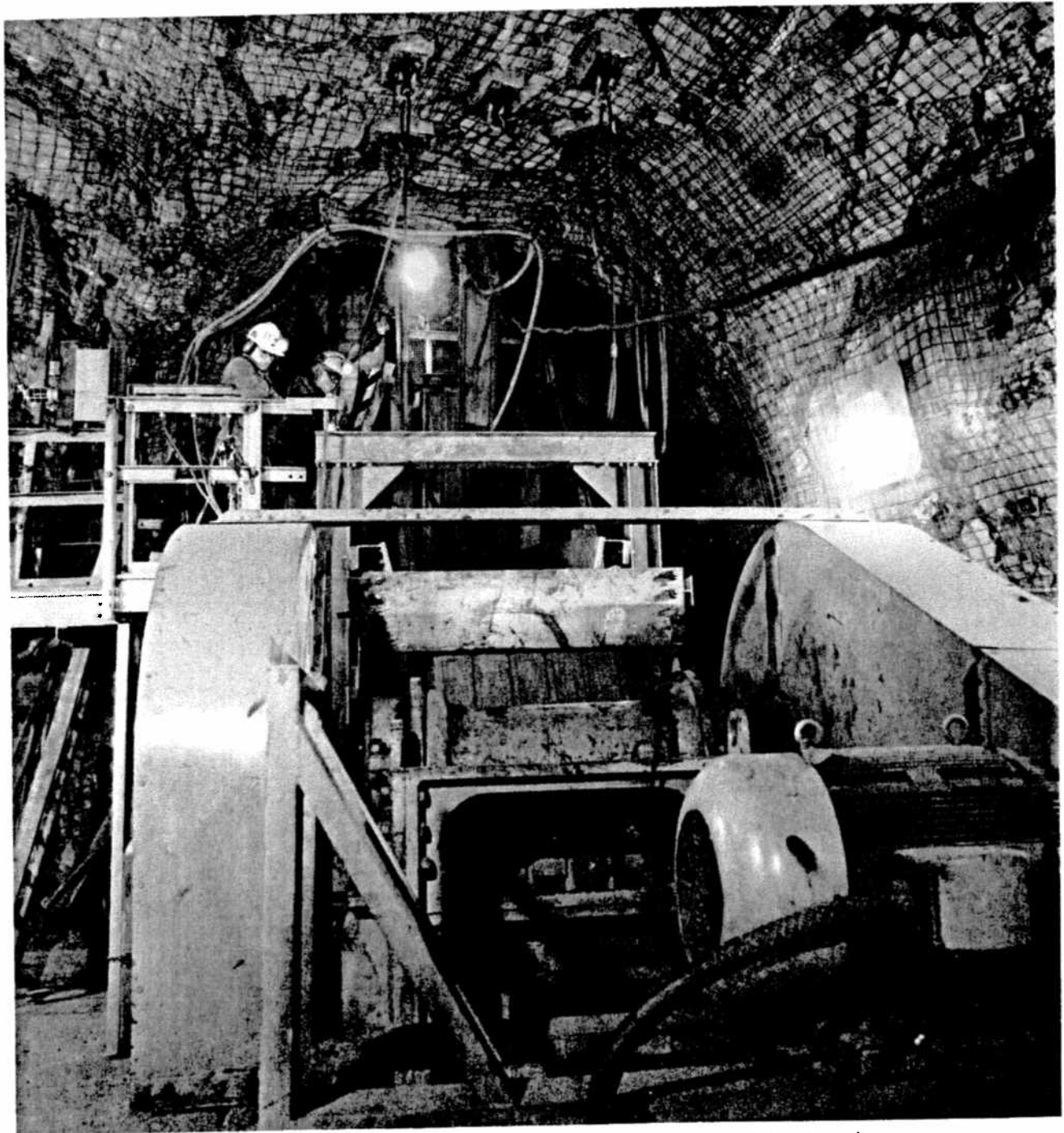
John Jeanveau, crusherman, left, and Rino Tessarolo, maintenance foreman, inspect the newly installed Eagle crusher.
