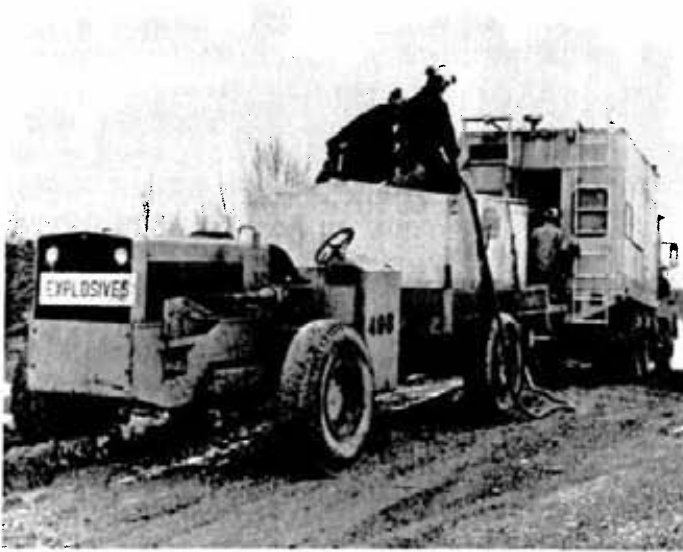
Tim Dupuis, mechanized slope driller, and Lawrence Caverly, construction leader, fill a hopper on the back of a scissor lift truck with the pumpable emulsion manufactured in a mobile plant. Gilbert Prieur, assistant plant operator for Ireco checks the progress at the mixing truck
