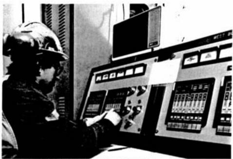
Smelter circuit operator Robert Guerin controls burners on the number two furnace through this computer.
