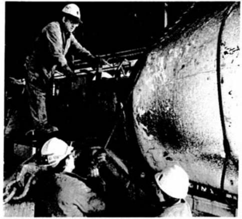
From left, maintenance mechanics Ron Vallancourt, John Laban and Glen Butcher guide a sling over the end of the hot metal car.
