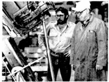
John Prudhomme, left, a machinist, checks the performance of a special jig he designed for sawing dog leg coolers with maintenance mechanic John McLaren who operates the horizontal cut off saw.
