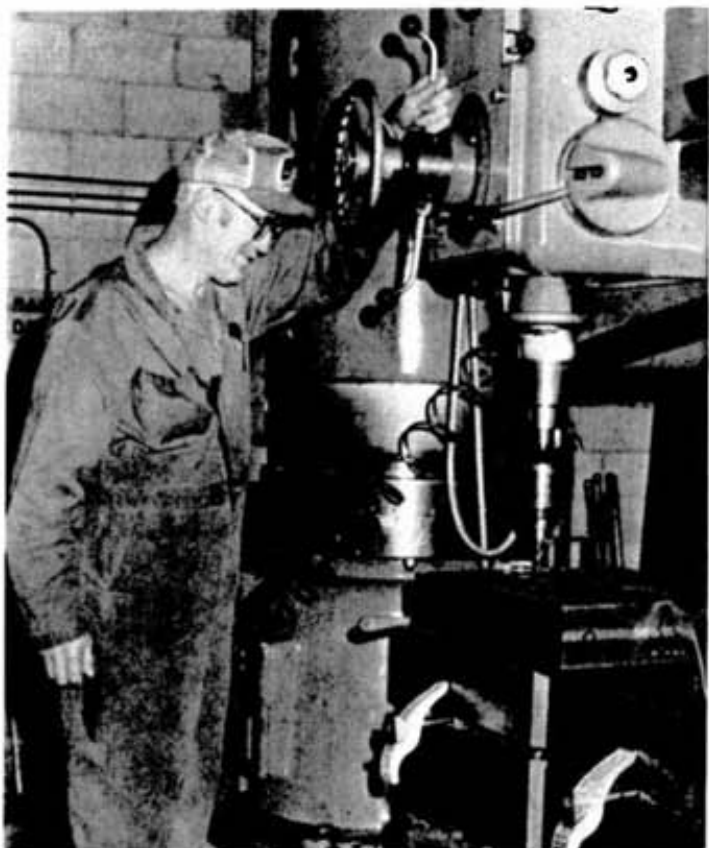
John Sioboda, maintenance mechanic, taps lifting holes in copper coolers on the radial arm drill with a high speed tapping attachment.
