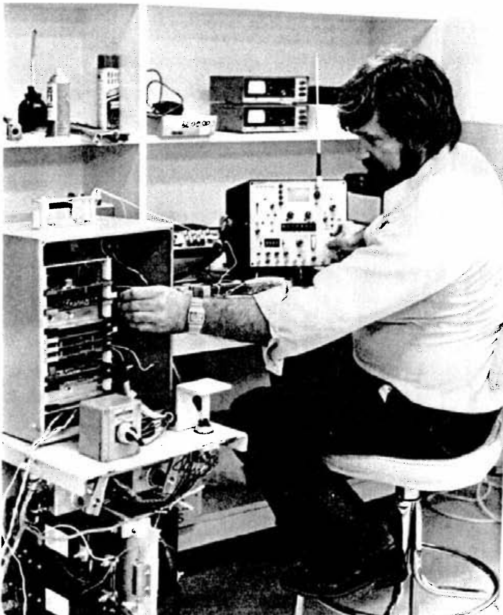
Richard Forget, instrumentation specialist, tests a prototype design for radio remote controlled machinery.
