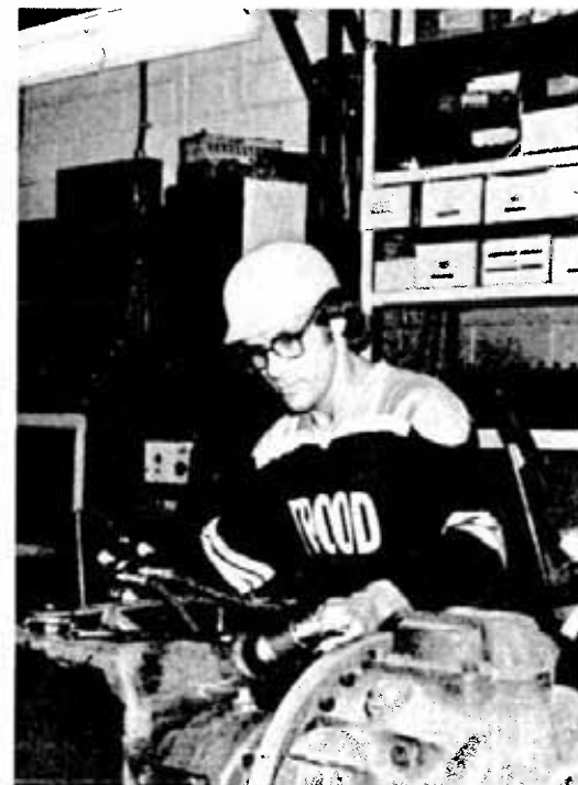
Ugo Crozzoli, rod repair inspector, checks for minute cracks in a rod with an ultraviolet light and magnetic coil.
