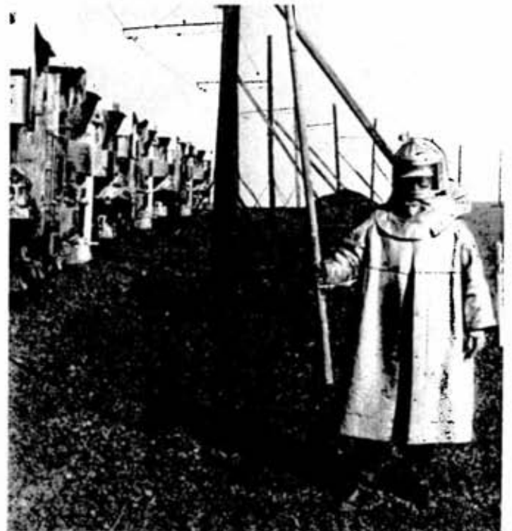
John Herman, slag dump leader, looks like a cross between a Martian and a Knight of the Round Table in the aluminized rayon outfit that protects him from the slag's heat. The train comes under his direction at the dumpsite. The slag dump leader decides at exactly what spot the slag will be dumped. Attached to the pole in his hand is the wire that energizes the slag pot's electrical dumping mechanism.
