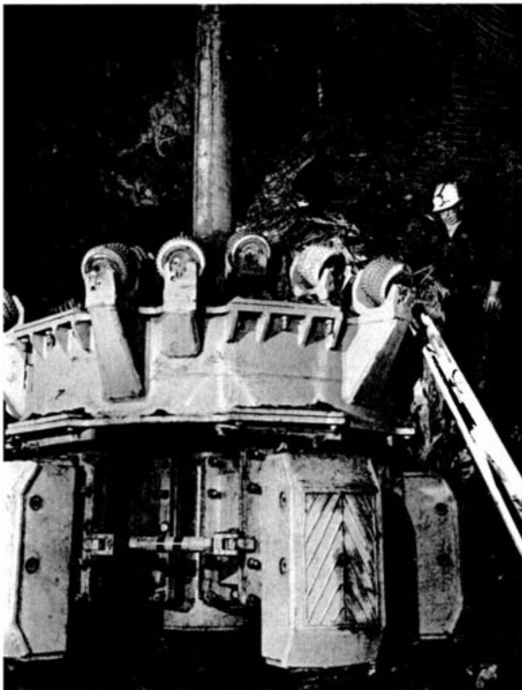
The raise bore head and its non-rotating stabilizer dwarf John Ernst as he inspects the apparatus.
