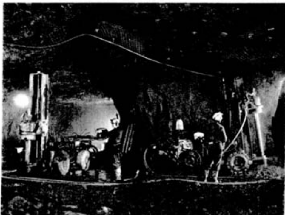
Claude Thibault, left, and Ron Storms operate a pair of Inco developed and manufactured In The Hole Drills at North mine. Designed by the mines research department these drills are extremely portable, much more compact, more efficient and more powerful than ITHs of older design.
