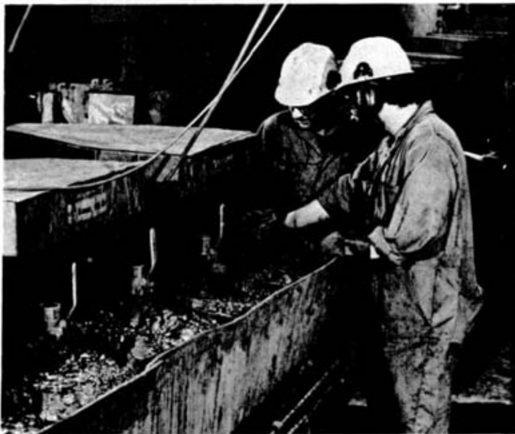
Senior process assistant Luc Bedard, left, and Dan Pelland, process assistant, make adjustments to a bank of flotation cells used in the course of a pilot plant campaign.
