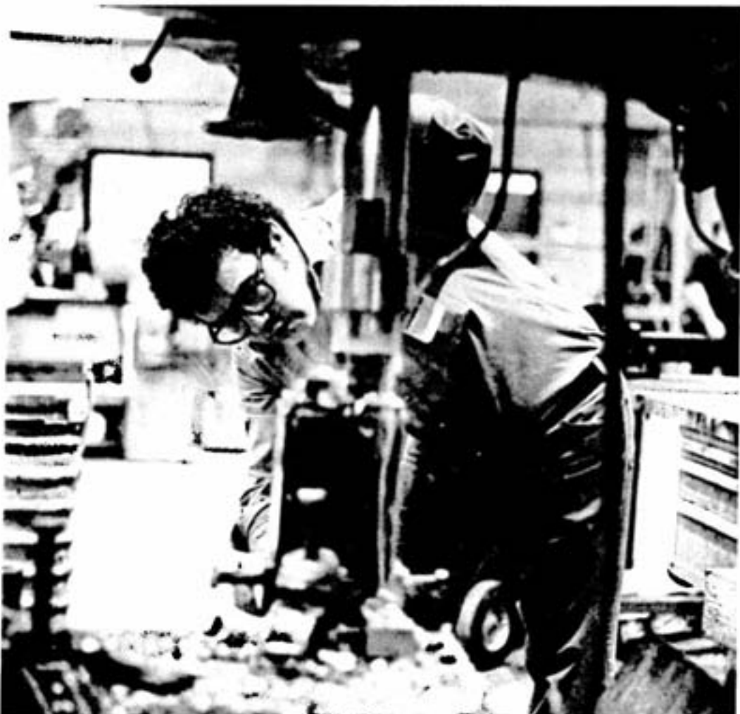
Maintenance mechanic Lou Fantasia files the burrs off the plug area of the copper jacket.
