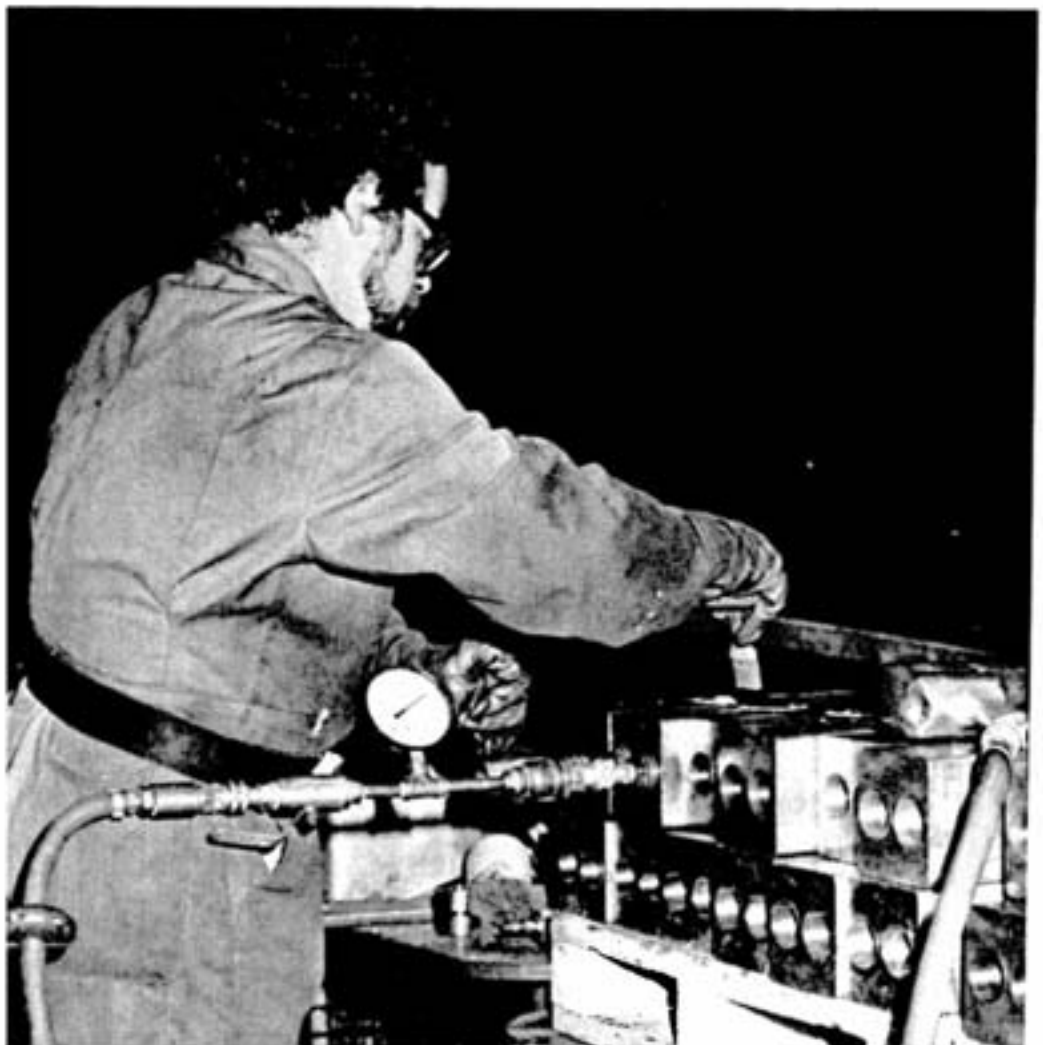
Maintenance mechanic Leo Bombardieri begins drilling an end hole in the copper cooling jacket.
