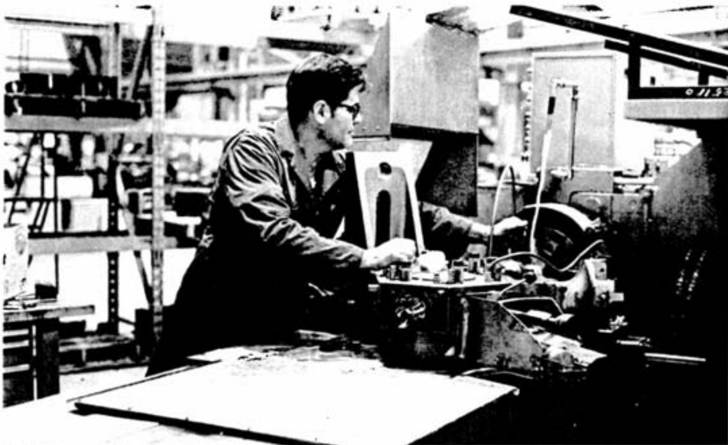
Dave Roberts, a machinist, sets material in the chuck of the NC lathe to manufacture a plug for the cooling jackets.
