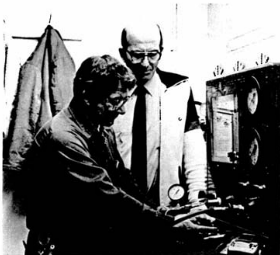
Larry Aubertin, repairman leader, left, tests a demand breathing apparatus regulator while centre supervisor Gene Dankewich looks on.
