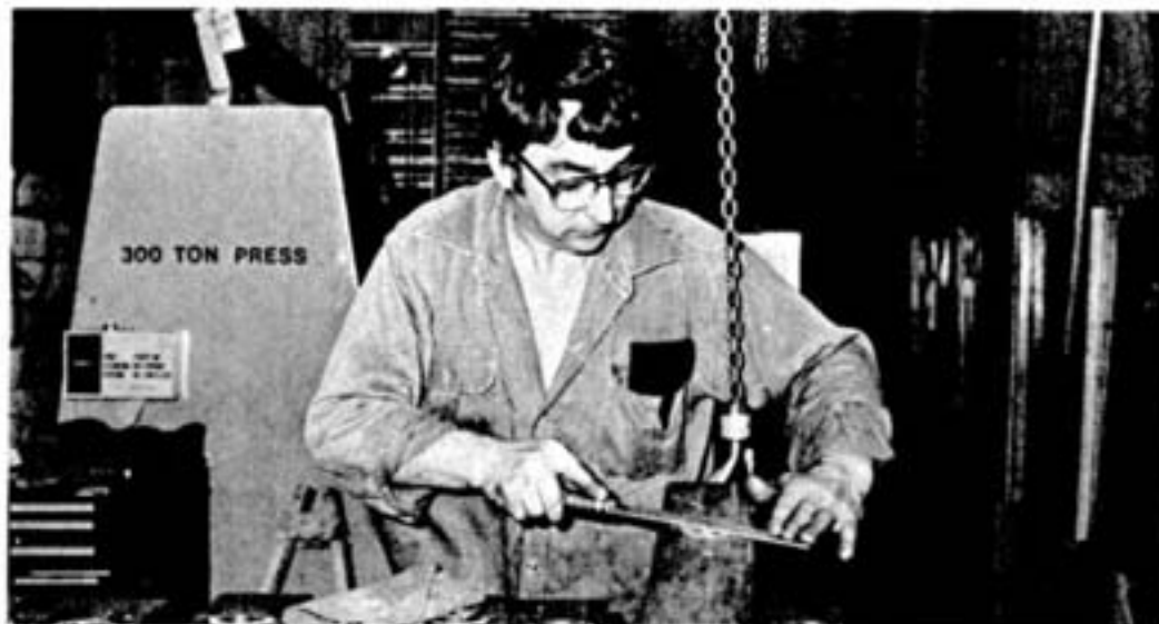
Maintenance mechanic Lou Fantasia files the burrs off the plug area of the copper jacket.
