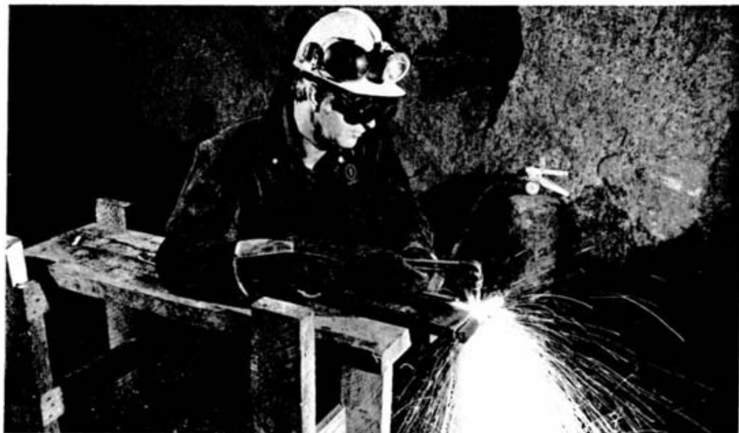
A school instructor at Stobie mine, Tom Bell, uses an acetylene torch to burn a piece of plate steel while on course.
