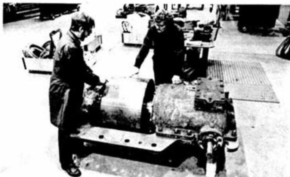
An assembled rotate drive gear box complete with shaft and other components looks like this.
