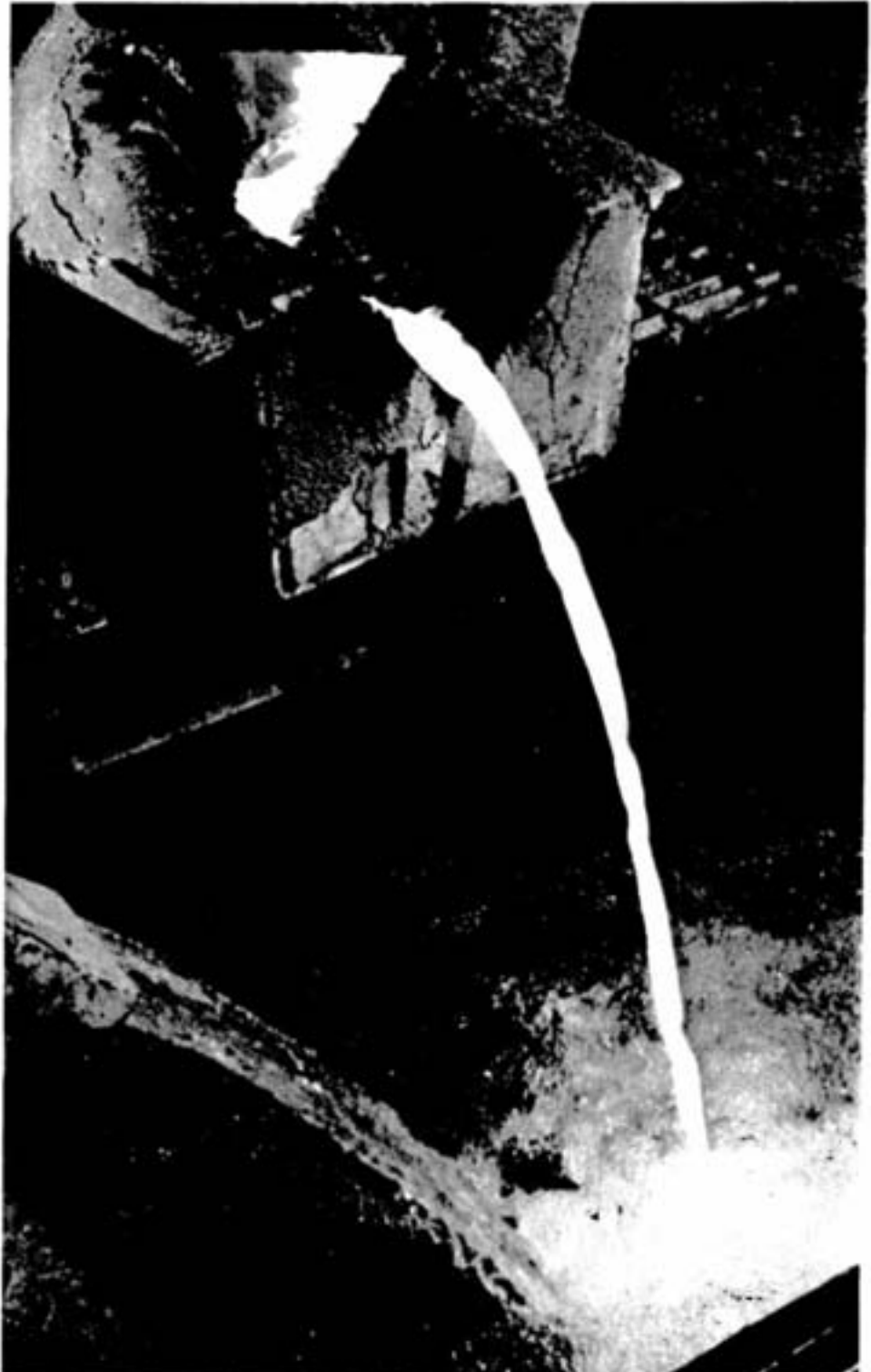
Utility nickel shot is formed when molten nickel hits a water spray and is broken into granules.
