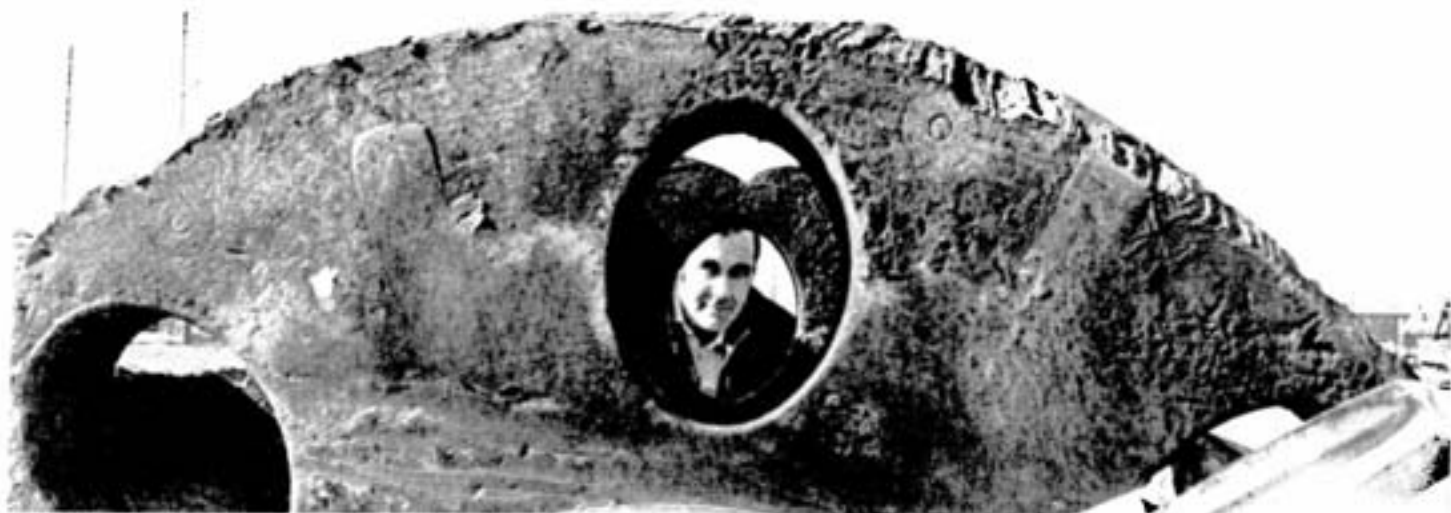
Bruce Warren points to the hollow construction of the old variety of trunnions and the cracks and other wear that it has suffered over the years of service supporting a kiln in the IORP.
