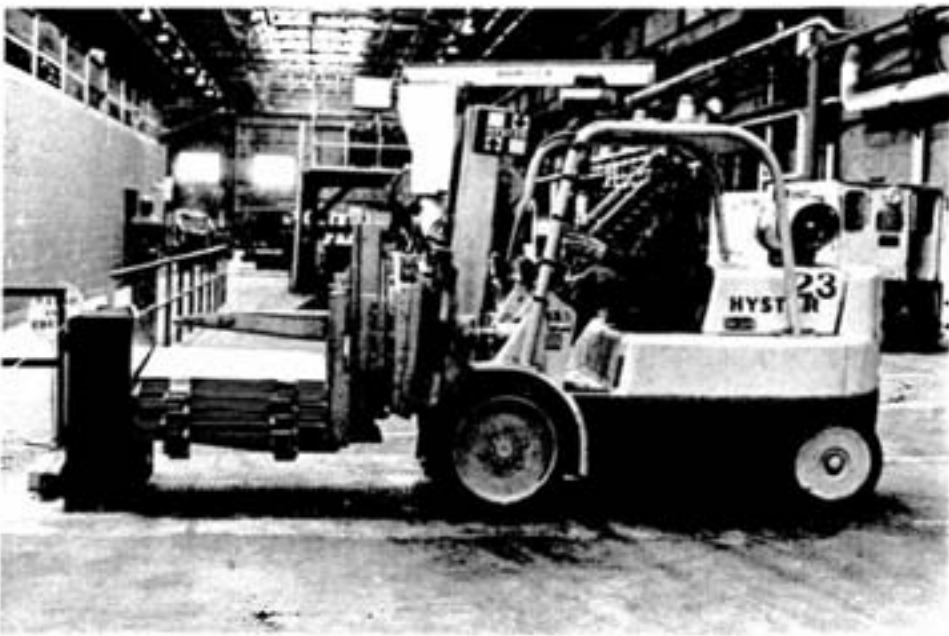
Cathode handler truck operator Army Bresolin straightens the cathodes against the bumping block.
