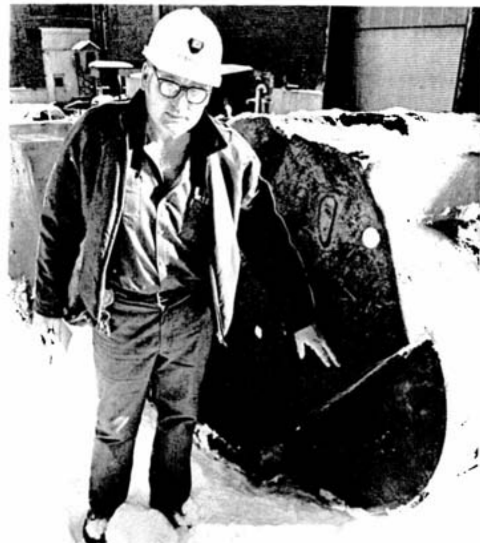
Enci DiFilippo, bucket shop foreman, assesses the wear on this bucket. Enci's final word is: the backside is torn off, a change of bosses and bushings needed, a new three piece cast lip required.
