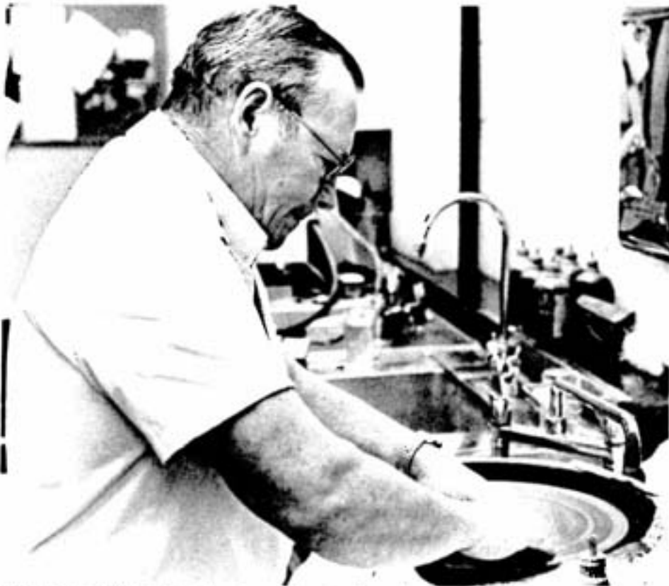
Norm York uses the cast iron lap to wear down the face of a thin section.
