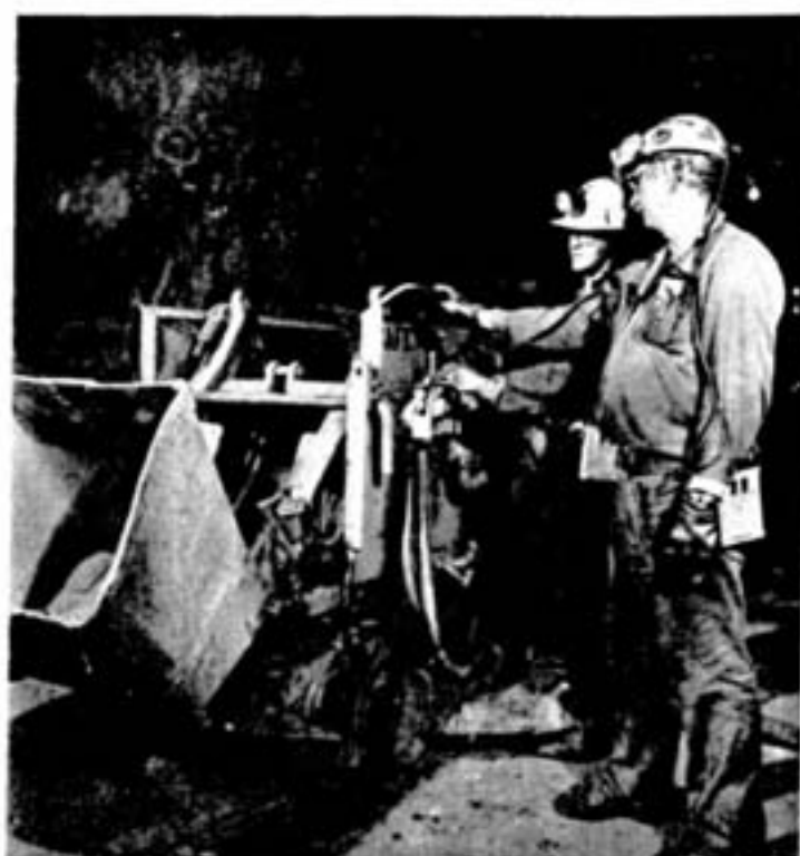
Training instructor Tom Bell, right, shows trainee Tom McPhail, how to operate a mucking machine.
