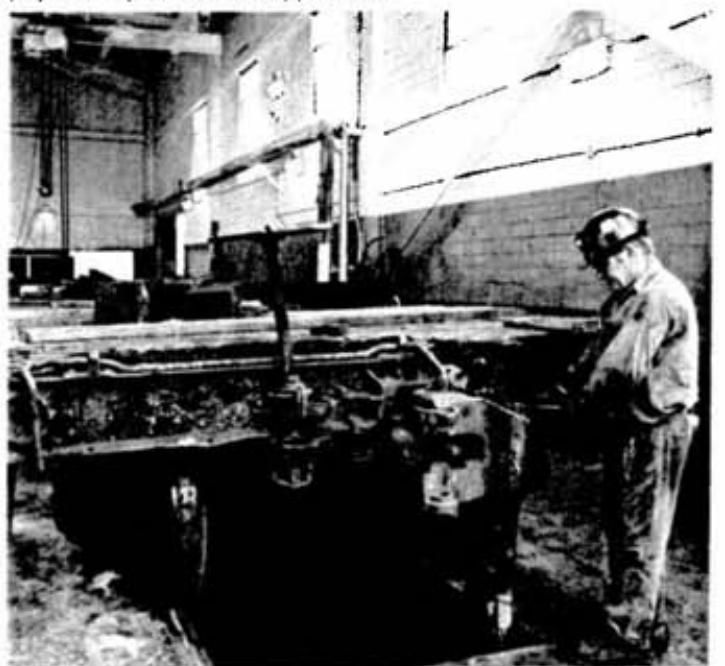
That's maintenance mechanic Gerald Wilson , checking an air valve on this flat car in the newly refurbished locomotive repair shop at Levack mine. In the foreground is the pit from which electricians service the locomotives and mechanics work under the cars when necessary. An overhead hoist provides plenty of lifting power.
