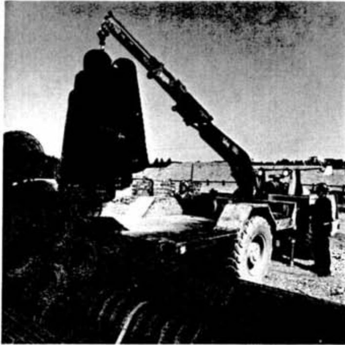
This is the new 5-ton boom truck which has recently been placed into service at the Levack West mine. Designed to handle supplies for underground workings, the unit here is being loaded with wire mesh screen. Lucien Belanger , left, a driller, signals to utility vehicle operator Fabian Harnett .
