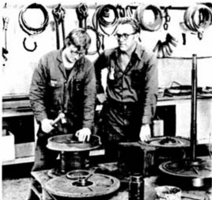
Raymond Poulin, left, and shop leader Bill Glogger fit a bearing in a slusher drum.
