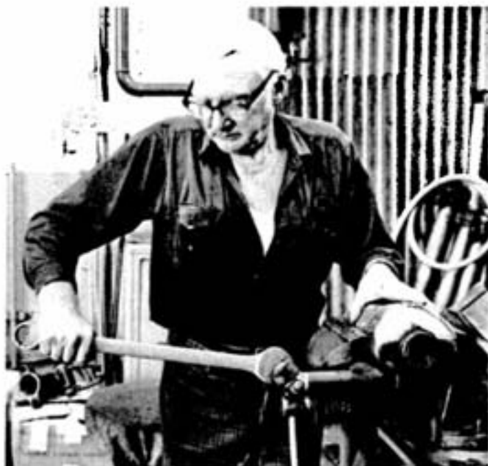
In the fully-equipped workshop, Bill Edkins repairs the muffler on a jackleg drill.
