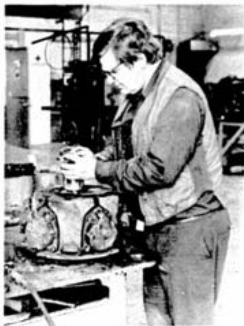
Norm Buchy repairs a chest valve for a slusher motor.
