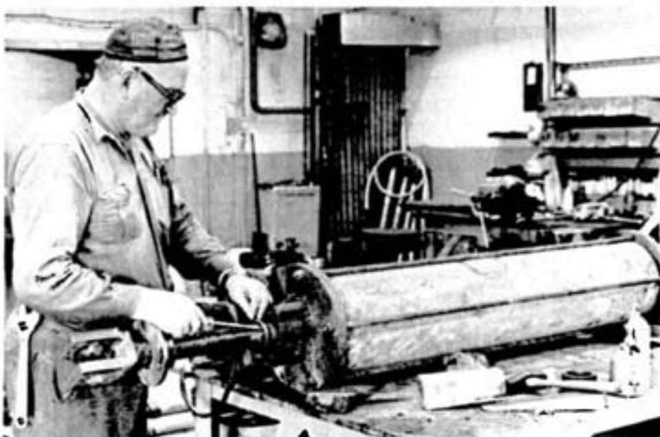
Bernard Cribbs packs an air cylinder before it is returned to the mining operations.
