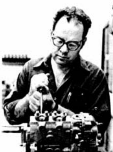
Sy Jean, garage mechanic, disassembles a fuel injection pump.
