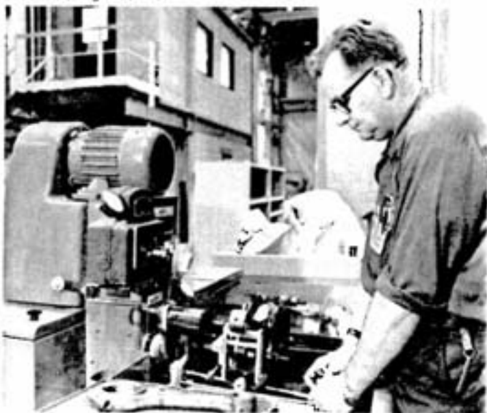
Garage mechanic Richard Lampman operates the connecting rod reconditioning machine.
