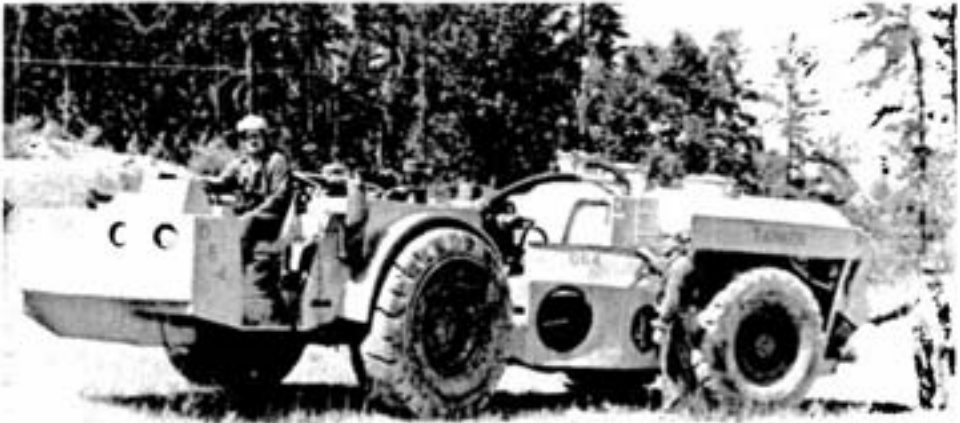
Were it not for the many innovative ideas put forth and developed by Inco personnel, this teletram, equipped with a large holding tank and a vacuum suction pump, would not be in service. Fabricated by the Levack West mine crew to clean up slimes from sumps and water from development headings, the unit underwent extensive testing before being sent underground. Teletram operator Armand Beaudry is shown at the helm of the new unit, with drillers Gerald Golden , centre, and Gerry Lappam attending the different controls.
