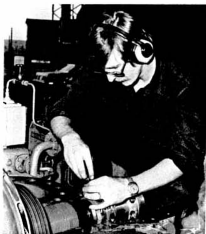
Terry Exworth carefully inspects the bearing on the Brown-Boveri blower shaft following extensive repair work.
