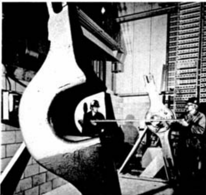
During installation of a 300-ton horizontal forcing press, second class machinist Vern Olson, left, holds a square while first class machinist Hans Fritzemeire checks alignment.
