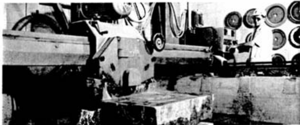
This semi-automatic diamond saw, valued at $35,000, can cut any block weighing up to 20 tons into any shape. That's Peter Ellero at the control panel, keeping a careful eye on the progress of the cutting blade.
