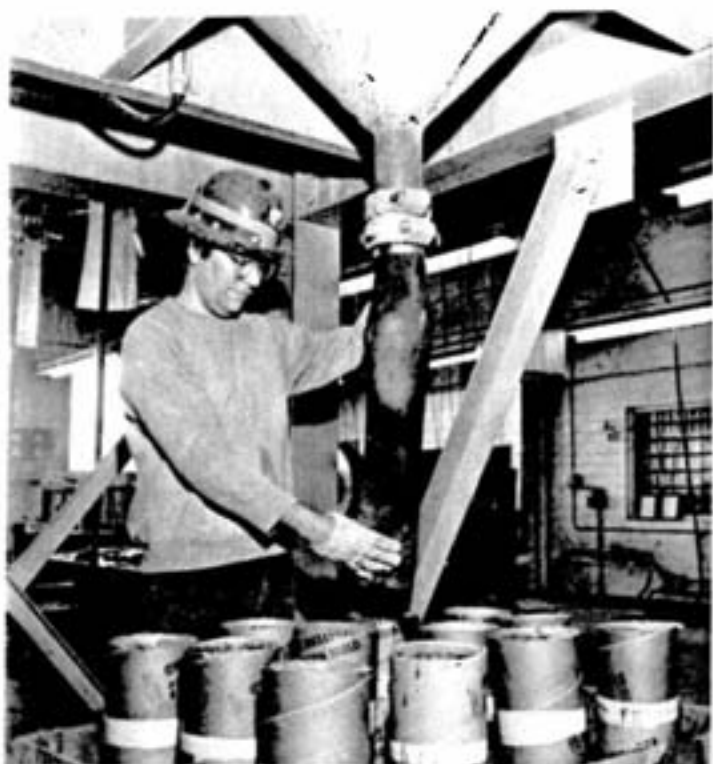
Don Desjardins, planner, fills test cylinders with a predetermined ratio of tailings, cement and slag.
