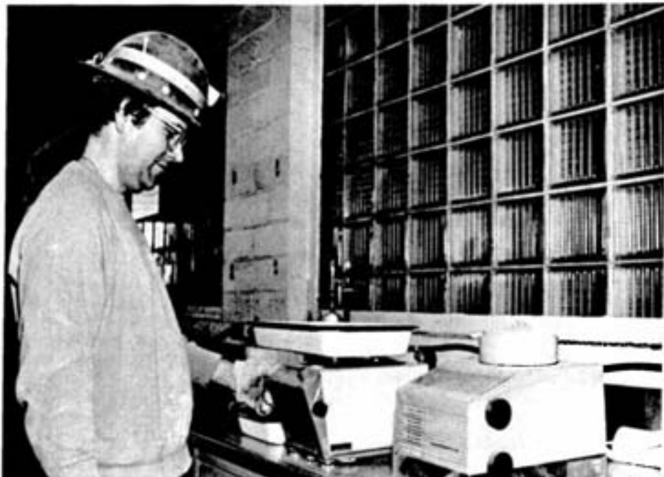
In the Murray mine sandfill research lab, planner Don Desjardins checks the moisture content of tailings brought in from an Inco sandplant.
