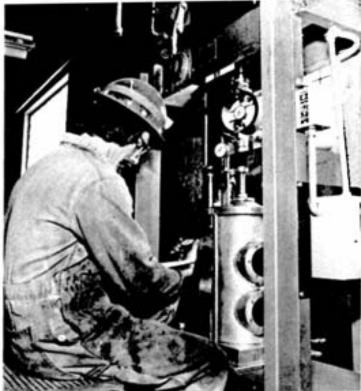
Project leader Dave Landriault takes readings from a tri-axial compression machine to learn the strength of a sample.
