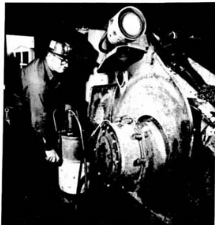
Ernie Arbour, first class garage mechanic, adds gear oil to the planetary of the wheel hub of an ST-2 scooptram, received from Garson mine.
