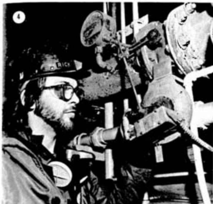
Rick McMahon, trainee, adjusts the ratio of natural gas and combustible air to give the required flame for the various phases of furnace operation.
