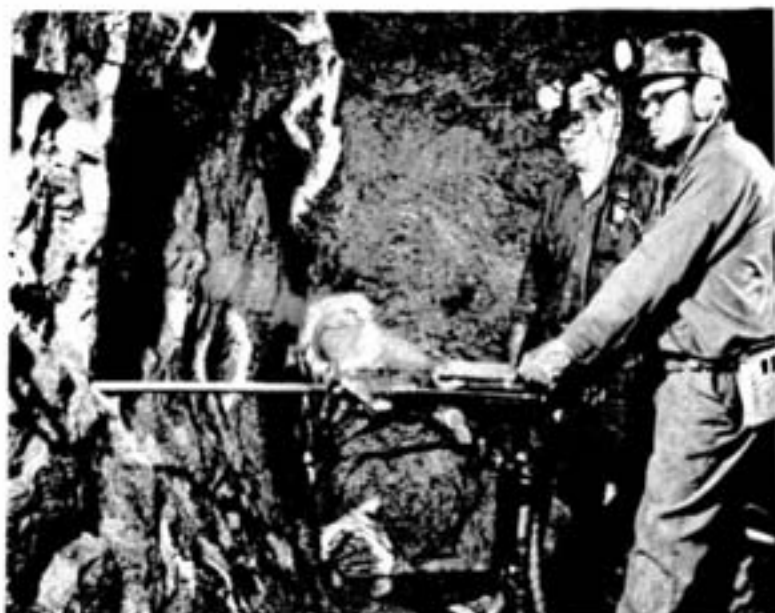
Hands-on training stimulates interest and provides confidence. Here, instructor Joe Grabish watches while trainee Dennis Menard drills slash with a jackleg drill.
