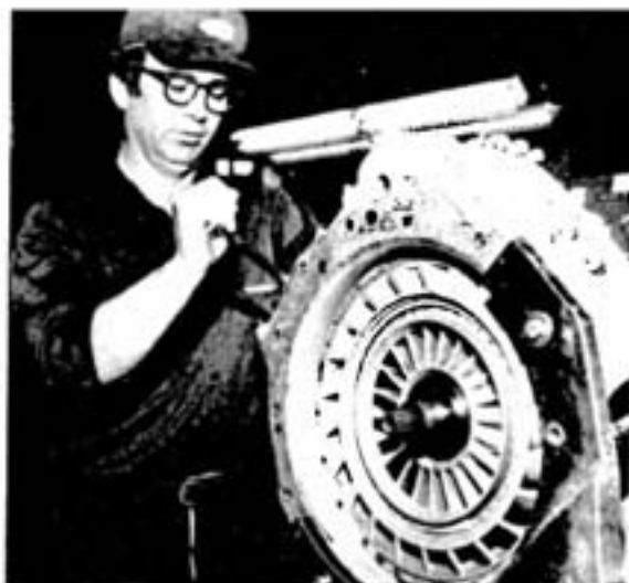
First-class garage mechanic Dennis Dowdall dismantles an FLT transmission from a Dorman diesel locomotive prior to repair.
