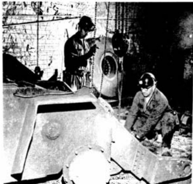
Rigger helper John Dutresne, left, and rigger leader Henry Prinoski dismantle the front section of a Jarco 130-A scooptram in preparation for loading onto a lowbed truck and subsequent tramping to the shaft for hoisting to surface in the cage.
