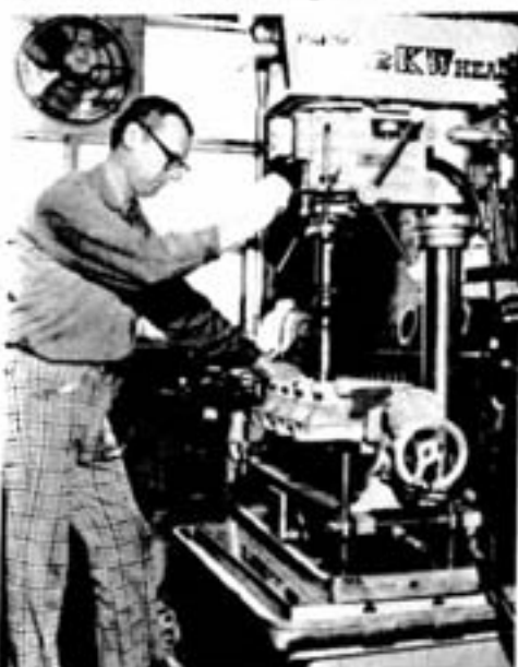
Steve Dominick, second-class garage mechanic, removes valve seats from the cylinder head of a diesel engine.
