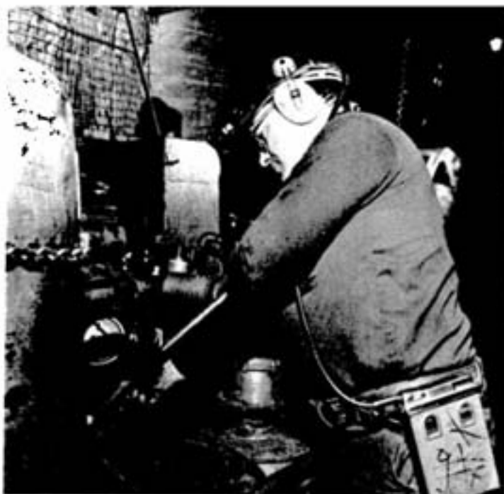
First-class garage mechanic Harold Reid repairs a scooptram's starter so the scoop can be driven into the garage at 2200 level. The scooptram will be used to move scoop parts previously dismantled.
