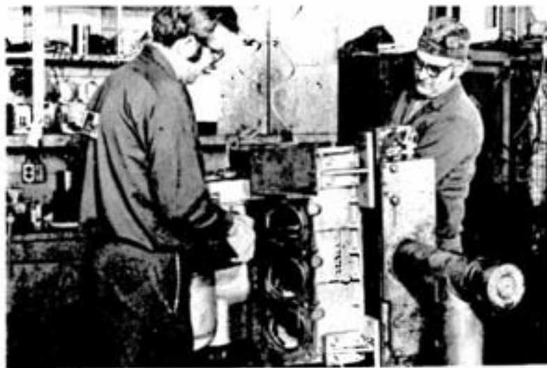
Vic Pregell, left, and Delphis Perrier, both first-class garage mechanics, replace a cylinder sleeve assembly in a Deutz engine block.
