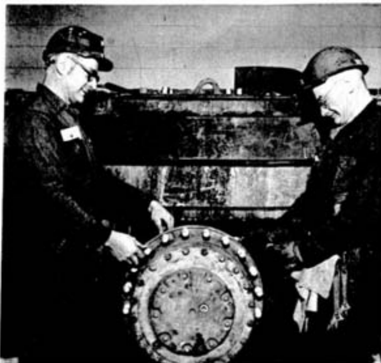
First-class garage mechanic Walter Hayduk, left, and first-class garage mechanic George Raymond change the studs on the rear wheels of a scooptram's engine section, which will then be shipped out for use at the Creighton mine complex.
