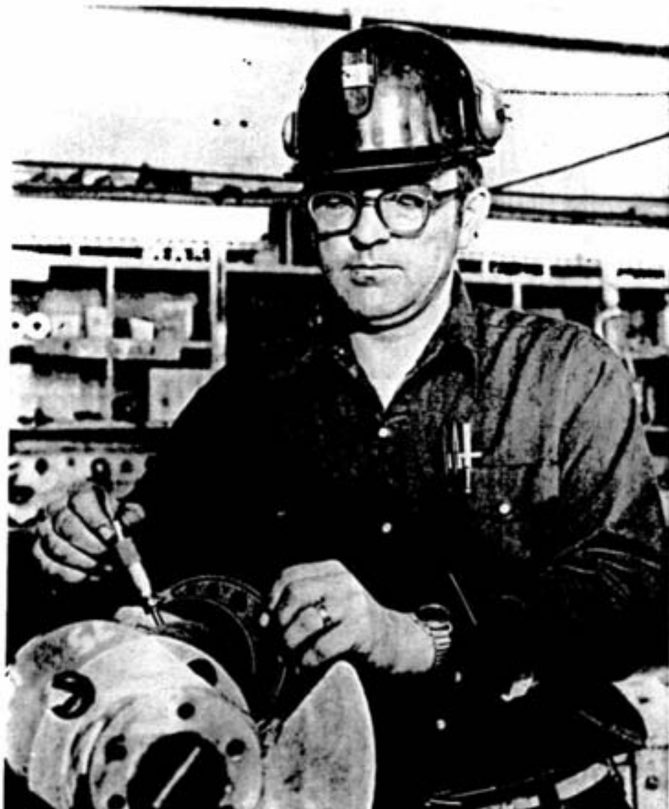
Pat Beaudry, garage mechanic leader, takes a metric micrometer reading on the crankshaft of a Deutz diesel engine.
