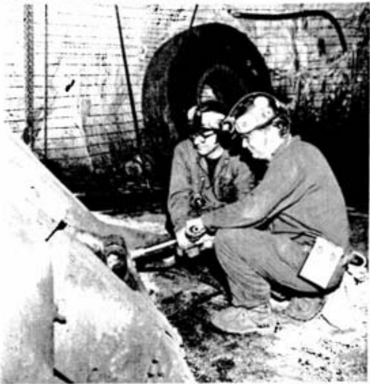
In the 1200 level garage, Garry Laforge, left, drill fitter, and Paul Blais, first-class garage mechanic, remove the T-bar from the front of a scooptram by using a one-inch air impact gun.
