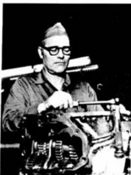
First-class garage mechanic Roland Lefebvre reassembles a Unimog 416 transmission following its repair.
