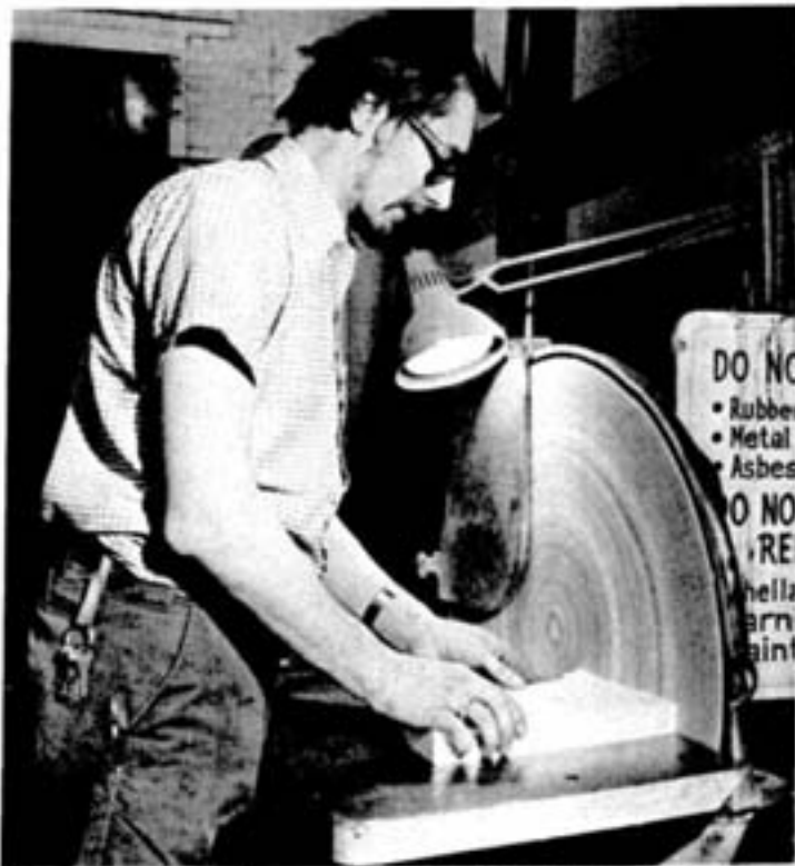
At the disc sander in the carpenter shop at the smelter complex, first-class patternmaker Allan Wuorinen prepares a pattern in wood for subsequent machining.
