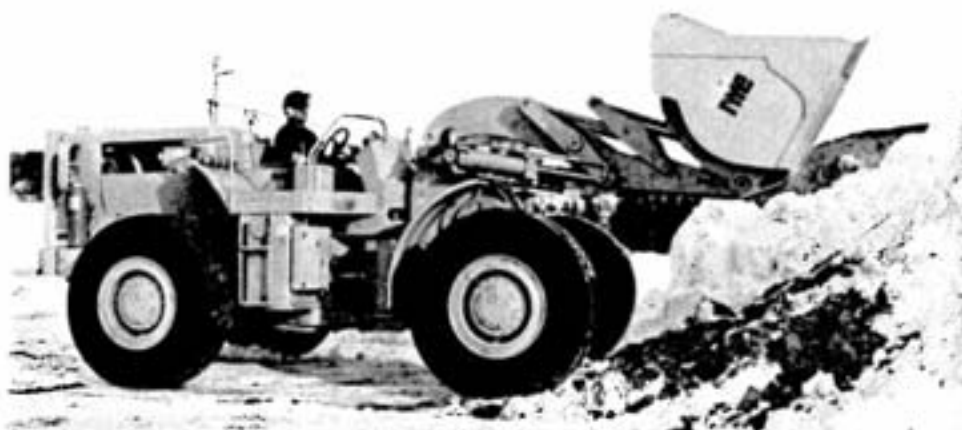
This is the specially-lowered Cat 966 front-end loader, recently supplied on a trial basis to the Levack West mine, where it will be used in a cut-and-fill and blasthole development application underground. The unit is fitted with a larger, 4 cubic-yard special mining bucket, smaller diameter 16:00 x 25 - 24-ply tires, rear end and fire protection system, no-spin differential and a lowered operator seating position. Below, Conrad Houle , left, Crothers marketing representative, points out the relocated, inclined console and tilting steering column to general mine foreman Glen Strutt and utility vehicle operator Eric Luttrell .
